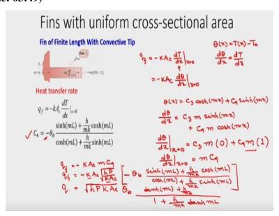
So we know that  $q_f$ , at x = 0, or at fin base is actually heat conducted to the fin and is equal to heat convected through the periphery of the fin surfaces and at the end of the fin surface because
