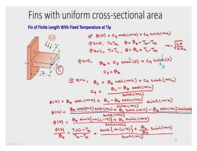
So now consider this fin of finite length and x we are measuring from the fin base and at the fin tip we have a specified temperature  $T_L$  okay, it may be connected to some liquid where it is maintaining the constant temperature. So that constant temperature is  $T_L$  we may consider.
