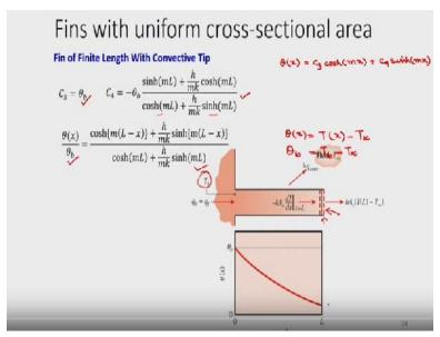
So for a fin of finite length with convective tip we have the equation as
