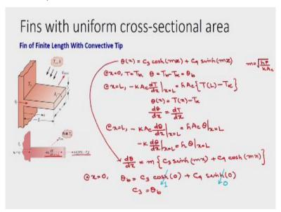
Now let us take the next case where we will consider fin with finite length with convective tip. So now we are seeing that from the tip also your heat loss is taking place due to convection. So in this case we have already discussed that the heat transfer or heat conduction through the fin will be equal to heat loss to the surrounding at the fin tip. So this is the case you can see here
