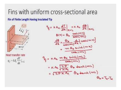
So if you consider that let us go to the next slide. Now you can see Fourier's Law we write  $-KA_c \frac{dT}{dx}$  okay, but as in this case x we have measured from the fin tip towards the fin base so it is a negative direction to the way your heat flux is there. So  $q_b$  or  $q_f$  is acting in the negative x direction that is why this minus, minus will be plus and we will write
