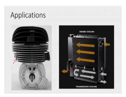
So you have seen the motor bike, right. So in the motor bike, just below the oil tank, you will find the engine of the motor bike and if you notice carefully, then you will find that in the engine there are some metal strips attached to that and these are the metal strips, where these metal strips are attached with the engine, which is cylinder. So combustion takes place inside the cylinder.
