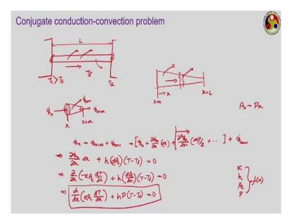
Let us take the situation where we have 2 plates, 2 surfaces rather. This surface is maintained at temperature  $T_1$ , this one is maintained at temperature  $T_2$  and these 2 surfaces are connected by a long solid bar or rod like this. So this bar is being subjected to temperature  $T_1$  at this end, temperature  $T_2$  at this end. Let us assume  $T_1$  greater than  $T_2$ , so there will be a conduction heat transfer in this direction.
