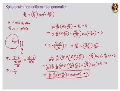
Let us quickly take care of one situation with non-uniform heat generation and for that, we are choosing a spherical geometry. We have not dealt spherical geometry in this week, that is
