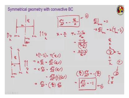
Let us see another situation of applying this boundary condition. Now our geometry, we are going to go for a symmetrical geometry in this case. Let us take Cartesian geometry only but a symmetrical one. That is we have a block, this is the centre line of the block, the coordinate starts from here. So this is identified at x = 0. Let us say the block is having a thickness of 2L.
