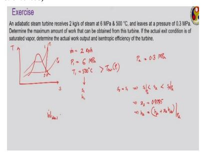
And now I would like to close up this by using the super-heated table. Here the question involves one of the adiabatic steam turbines. Let us try to do it very quickly, here let me draw that *TS* diagram of this. Here the initial state, here mass flow rate is given as:
