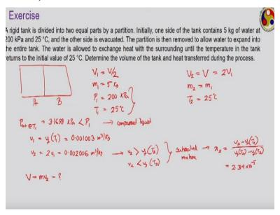
I would like to wrap up this by solving couple of numerical problems quickly. I have a problem here please read it quickly. Here you are talking about the rigid tank which is divided into two equal parts by a partition. So, we have our tank which is divided into two equal parts so this is your part A and this is your part B which are having equal volume. Initially one side of the tank is contents 5 kg of water at 200 kPa and 25 °C.
