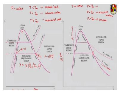
And that is exactly what we have here, we have a saturated liquid line which is exactly the locus of all the saturated liquid state. We have a saturated vapor line which is the locus of all the saturated vapor state and they are connected at the critical point. On the left-hand side of this dome like structure we call it compressed liquid, on the right-hand side we call it the superheated vapor and inside we have a saturated liquid-vapor mixture.
