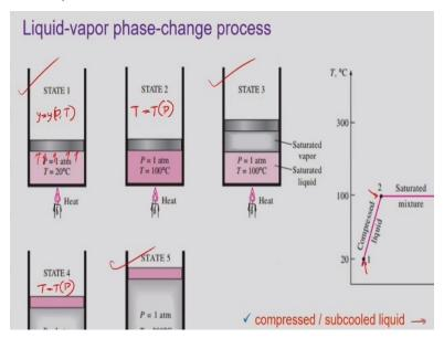
To understand the liquid-vapor phase-change process, we shall be talking about a simple experiment. In this experiment we have a piston cylinder arrangement, the piston is allowed to move such that it inside the atmospheric pressure is always maintained. So, to start with outside the piston it is open to atmosphere inside we have 1 atmospheric pressure and 20 °C temperature.
