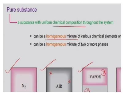
If pure substance refers to a substance which is having a uniform chemical composition throughout the thermodynamic system, i.e., the chemical composition has to be uniform and that is a very important term to have. We are not talking about difference in terms of its physical shape, difference in terms of its phase, but we are talking about difference in terms of chemical composition or I should say uniformity in terms of chemical composition.
