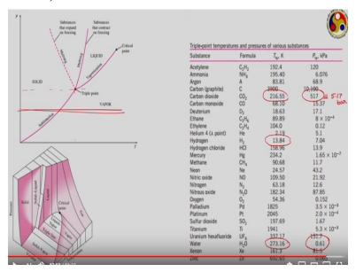
So, you can clearly see on this PT plane that three phases solid, liquid and vapor. And on the such PT diagram the triple line contracts to a single point which is called a triple point. It is again a unique characteristic of any system quite similar to that critical point.
