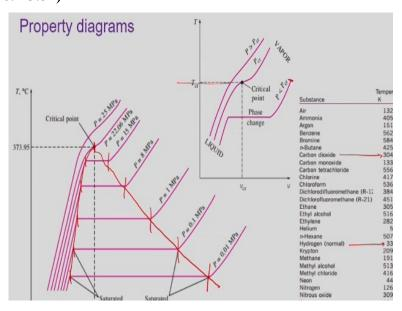
Now earlier we have drawn the Tv diagram only for a single case which was for atmospheric pressure are 0.1 MPa and here we have seen that initially we have a compressed liquid zone during which temperature increases rapidly along with the specific volume and then we reach the saturation temperature. So, this is the saturation temperature from this point we have the phase
