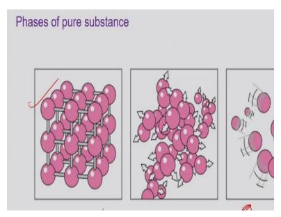
Pure substances can exist in commonly three different phases as we all know solid, liquid and gases. In solid, we generally have fixed lattice structure where all the molecules are bound in a ties lattice unit with maintaining a constant average distance between the neighbouring molecules these molecules can vibrate with respect to their own position but they cannot have translational motion.
