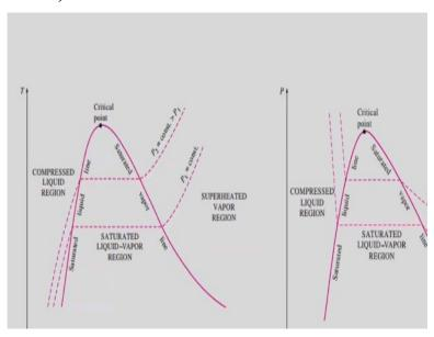
So, these are the two common property diagrams where we generally plot the phase change processes. If I just go back, you can see for each of the pressure levels now you are getting a saturated liquid point and a saturated vapor point. So, if we join all the saturated liquid points, till the critical point then we should be getting a line which is called the saturated liquid line.
