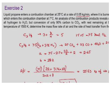
It is burned with 50% excess air which enters the combustion chamber at 7  $^{0}$ C. So, combustion product analysis has been done. It is shown that complete conversion of all hydrogen to  $H_{2}O$ , but combustion of only 90 % of carbon to  $CO_{2}$  with rest remaining at CO. Taking a gas exit temperature of 1500 K, we have to define the mass flow rate of air and the rate of heat transfer from the combustor.
