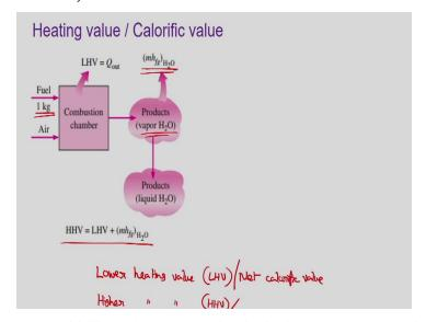
The final one that I would like to incorporate that is the heating value or calorific value, the name probably you have already heard, it refers to the amount of energy that we can get by complete combustion of 1 kg of fuel. The previous two definitions are on molar basis this is on mass basis. If we burn 1 kg of fuel and we have complete combustion, then amount of energy that is released is called the heating value or calorific value.
