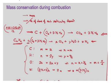
Now one important thing is that during the combustion process the mass has to be conserved. Of course, here we are neglecting the theory of relativity that is a conversion of mass to energy because that is applicable only during or that is significant only during the nuclear reactions. Here one thing you have to keep in mind that whenever we are having some kind
