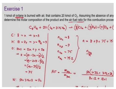
Now here we have one numerical exercise to deal with. The problem involves 1 kmol of octane, it is burned in air that contains 20 kmol of oxygen. Assuming the absence of any reverse reaction, so we are assuming there is no reverse reaction, there is no dissociation. So, the carbon dioxide and water vapour produced during the combustion reactions they are not breaking back to their constituents.
