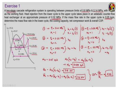
Let us now take a numerical example just to see how we can deal with this cascaded refrigeration system. And I should mention that here though we have talked about two-stage but it is possible that we can have more than two stages also, three or four stages are also very much possible, particularly when we are looking to go for very low like cryogenic level temperatures. Now in this
