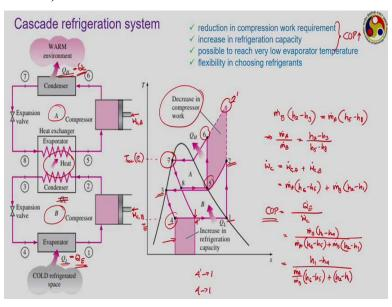
The cascade refrigeration system, where not one but rather we have two refrigeration cycles. quite similar to the combined cycle that we have discussed earlier in conjunction in the power cycles. It is also something like combined cycle used for refrigeration purposes. Here just look at the bottom cycle given by this B, this bottom cycle is picking up the heat from the cold refrigerated space  $Q_{in}$
