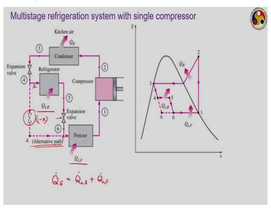
We can have a few other designs also. Like this is a multi-stage refrigeration system with single compressor. This is something that we have actually in our domestic refrigerators. Remember in your domestic refrigerators, we are actually in need of two different temperature levels. Like the common food stuffs, fruits, vegetables that we store in a normal refrigeration compartment, there
