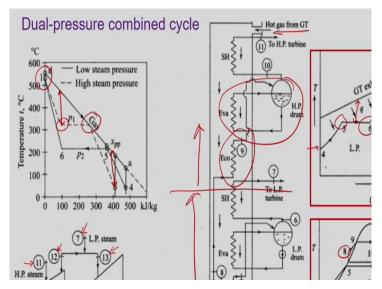
Now the dual pressure combined cycle is something that requires a very brief mention. Just look at this diagram where we are having temperature on the vertical axis and amount of heat transfer in the horizontal axis. This continuous line represents the gas. As it is passing through HRSG it is continuously losing the temperature where it is supplying energy to the steam. Now there are two stream lines shown one at low pressure and other at high pressure.
