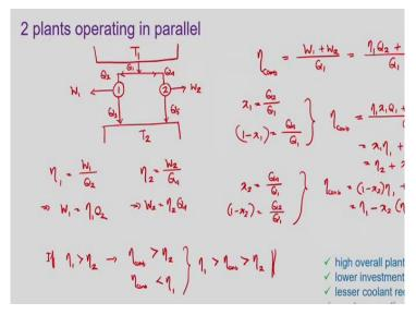
We have a temperature reservoir operating at temperature  $T_I$ , another operating at temperature  $T_2$  and we have two plants: this is 1 and this is 2. They are operating in parallel that means both are receiving energy from the same reservoir  $T_I$ . Let us say  $Q_I$  is the total amount of energy being extracted from this out of that  $Q_2$  is going to the first one which is rejecting  $Q_3$  to this  $T_2$  reservoir and producing  $W_I$  amount of work.
