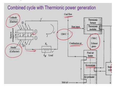
Another quite potent option is thermionic power generation. When we heat certain material beyond certain temperature that can emit electron. That is something we will refer as thermionic power generation. Generally, metals when they are heated to a temperature beyond the threshold, free electron starts coming out of this. So, this material is called cathode and also emitter which rejects these electrons and then we have an anode or collector where these electrons are collected.
