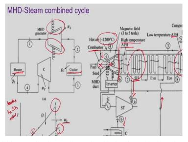
Now we would like to talk about a few other kinds of combined-cycles. As I have just mentioned and I shall be talking about three innovative approaches very quickly. And the first one of them is MHD. MHD refers to magneto hydrodynamic generator: M for magneto, H for hydro and D for dynamic generator. Here the idea is very interesting you know that from Avogadro's principle that whenever a conductor moves in a magnetic field, we have electricity generation.
