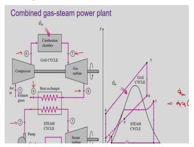
So, this is what we are talking about. There are several kinds of combined cycle plant, the common choices for the topping cycle and bottoming cycle or I should say the combination of topping cycle in bottoming cycle can give you different conceptual design of combined cycles. But the most common combination is the one that you are talking about is a gas turbine as the topping cycle and steam turbine as the bottoming cycle.
