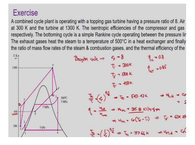
A combined cycle plant is operating with the topping gas turbine having a pressure ratio of 8. Air enters the compressor at 300 K and turbine at 1300 K. Isentropic efficiencies for the compressor is 80% and gas turbine is 85%. Bottoming cycle is a simple Rankine cycle operating between the pressure limits of 7 MPa and 5 kPa.
