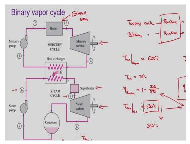
The term binary of course refers to two and by now you already know that we have a topping cycle. Let me write this side detail utilisation of the space. We have topping cycle which is of course a Rankine cycle and working with mercury as the working medium.
