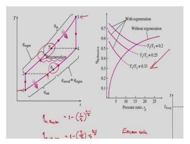
So, this is how a practical regenerator works where, we have 1-2 here of course, we are not considering the irreversibilities inside the turbine and compressor. That is, we are taking isentropic efficiency of both compressor and turbine to be equal to 1. Then 1-2 is a compression process 2-5 is the regeneration process, regeneration for air heating then 5-3 refers to the combustion process.
