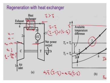
Regeneration plus another heat exchanger, which is called the regenerator. The idea is that the energy of the exhaust gas coming out of the turbine will be utilised to preheat the air before it is allowed to go to the combustion chamber. Like we have seen with the use of reheater, the exhaust gas temperature can be very, very high. Even though there is no reheater, size of temperature will be quite significantly higher compared to the air temperature coming out of the compressor.
