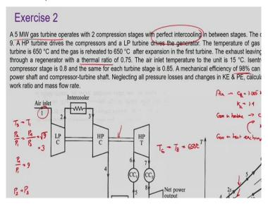
I am giving the diagram first so that you can directly compare the diagram. Here we have 5 MW gas turbine plant. It is operating with two compression stages, so this is the LP compression stage and this is the HP compression stage and perfect intercooling in between the stages. So, you are having perfect intercooling that is once it is perfect intercooling, so we can easily say that:
