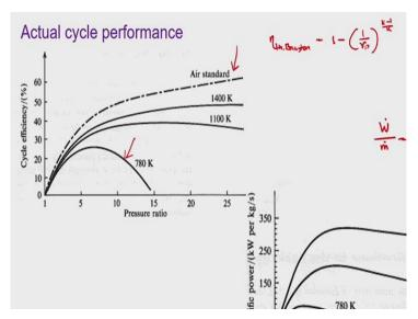
But before that just check out the actual cycle graphs. This is the variation of cycle efficiency with pressure ratio. The dotted line is the air standard one which follows the analysis that we have done yesterday. Because we know that the thermal efficiency for Brayton cycle is:
