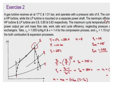
Let us solve another numerical problem to use the same concept of high pressure and low-pressure turbines. So, here we have a gas turbine which is receiving air at 70 °C and 1.01 bar
