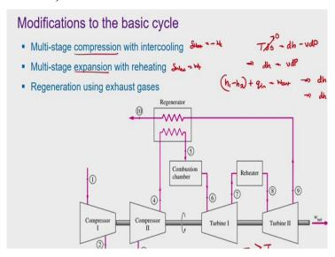
Now let us move to the modifications in the basic cycle. We have seen that back work ratio can be quite significant. Of course, in this case the back work ratio is smaller but in practical cases back work ratio can be in the range of 40-50-60%. And therefore we need to make certain kind of modification in the basic cycle so that we can increase the work ratio or we can reduce the compressor work requirement.
