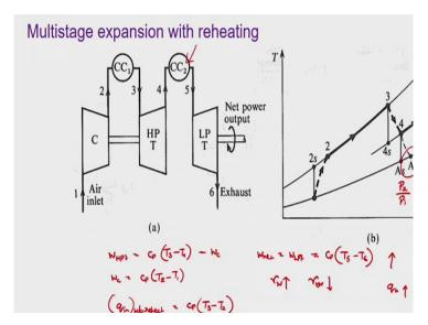
The opposite of intercooling is multi-stage expansion with reheating. Because of the same reason just to increase the specific volume, we can separate the turbines into 2 stages. Look at it is quite similar to the power turbine that you have shown here. The HP stage of expansion is mounted on the same shaft as the compressor but the LP stage is separate which is mounted or on the same shaft as the generator.
