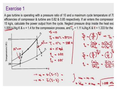
Now let us see what we have as an effect of the isentropic efficiencies. Here we have a gas turbine operating with the pressure ratio of 10 and a maximum temperature of 700  $^{0}$ C. Isentropic efficiencies for compressor and turbine are given and they are separate in this case. Air enters the compressor at 15  $^{0}$ C at a rate of 15 kg/s, so you calculate the power output.
