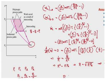
So, work input requirement for stage A, 1-A:
