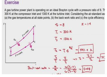
An ideal Brayton cycle is just this that is both compression and expansion processes are isentropic and there is no pressure drop anywhere in the cycle. So, just read the problem here the pressure ratio is 8 so we have
