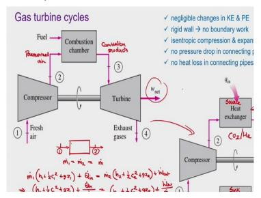
So, this is a typical open cycle kind of gas turbine where we are supplying fresh air in a compressor first. There this air is compressed to a much higher-pressure level and also temperature increases simultaneously. Now this high-pressure air is taken to the combustion chamber where you are also spraying the liquid fuel inside the combustion chamber. When combustion happens thermal energy is released and this high temperature combustion gases are subsequently taken to the turbine.
