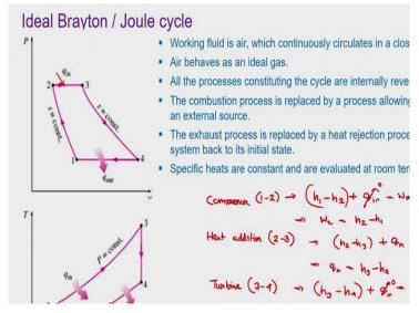
Now this is the ideal cycle that I am talking about which is called the Brayton cycle or Joule cycle. Brayton cycle is the most common name and therefore shall be sticking to that. Look at the processes there plot on Pv and Ts diagrams are shown. Here 1 to 2 is an isentropic compression process which is being done inside the compressor. Then 2 to 3 is a constant pressure heat addition process. Just going back to the previous one, let us try to get the cycles or nature of the processes from here.
