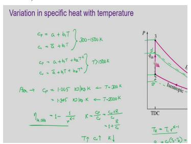
The next factor i.e., the variation in specific heat with temperature. This is something that we can directly represent on the cycles. Specific heats are strong functions of temperature. When we are talking about lower temperature say something in the range of 300 to 1500 K, it is generally:
