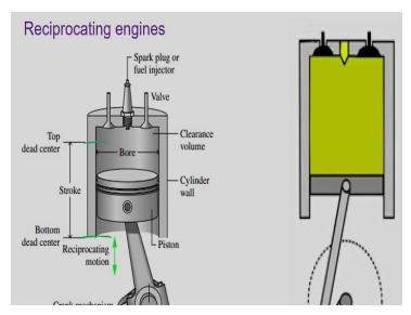
These are some diagrams which have shown in the previous week itself. This is standard reciprocating engine for we know that the piston reciprocates within the cylinder. Generally, the top most position is referred as the top dead centre and the bottom most position refers to the bottom dead centre. This is the top dead centre position and this is the bottom dead centre position and the distance between the dead centres is called the stroke volume or displacement volume.
