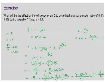
What is the effect on the efficiency of Otto cycle having a compression ratio of 8,  $c_v$  increases by 1.6 % during operation k equal to 1.4 that is given. Only the variation of specific heat that we have to consider or variation of k with  $c_v$  that you consider to get the cycle efficiency. Now for Otto cycle we know that,
