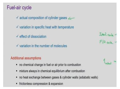
Fuel-air cycle is a modification of the ideal cycles where among all the factors that I just listed in the previous slide not all but four of the factors we are considering or we are adding to the actual cycle. Factor number 1, the actual composition of cylinder gases: in fuel-air cycle just I repeat we are adding these factors to the ideal cycle which we have already discussed. Like the Otto and Diesel cycle that we have discussed in the previous week.
