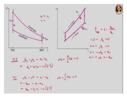
The same Pv diagram shown here, so we can see there are four processes: two isentropic processes and two constant volume processes. The same thing shown on a Ts diagram 1 to 2 isentropic processes, entropy is constant is the vertical line, same applies to 3 to 4. But during 1 to 2, temperature increases during 3 to 4 temperature decreases and 2 to 3 and 4 to 1 are constant volume processes.
