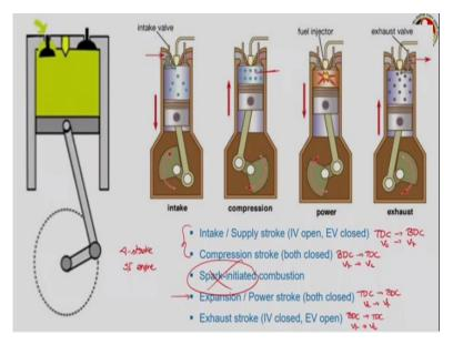
Now, let us see how a reciprocating engine works. Here I have a small animation taking from YouTube. Just look at this, this is the piston then, this is your inlet valve through which the fuel will be allowed to come in, this the exhaust valve through which the exhaust gas will be going out, this is your spark plug. So, initially when the piston is at the top dead centre somewhere here, both the valves are closed.
