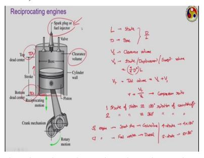
Now, we come to the reciprocating engines, reciprocating engines are the application zones of this gas power cycles or air standard cycles. Just as very simplest schematic diagram of reciprocating engines is shown. Here we have piston so, this is the wall of the cylinder inside which we have this piston having circular cross section as shown in the diagram. This piston can move up and down inside the cylinder to facilitate such kind of reciprocating motion, we have the crank mechanism.
