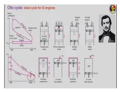
So, the cycle that we have to consider here is called the Otto cycle which is the ideal cycle for SI engine, conceptualised first by Nicholas Otto, the Frenchman. See, this is the ideal scenario or I should say the actual scenario. We have a compression stroke then, power stroke, exhaust stroke and intake stroke, going on in cycle and also between compression power stroke, we have the combustion process by spark.
