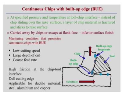
Now there is one situation, continuous chip with built-up edge. So they are specified that particular pressure and temperature that situation that what way the chip and tool interact, that instead of the chip sliding over that rake phase, there is a possibility of the chip chipping on the rake phase and of course a layer of the chip material is fracture and stick to the rake surfaces. So that kind of situation we can see that this kind of material is generated.
