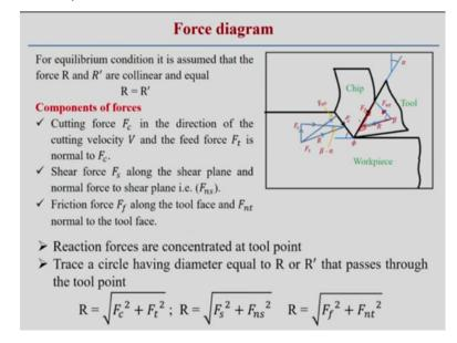
Now if you see, here from the tool site, this frictional force is there and this is the normal force and that this is a resultant force R. These 3 forces are acting. If you look into the body with respect to the tool, then from the work piece part we can see there is a shear force is acting here and Fs we define the shear force Fs on the shear plane, it is acting shear force and normal to that normal force and resultant of this is basically R, shear force and this.
