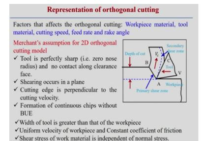
Now in orthogonal, we analysed the chip formation all these things, but what we look into the orthogonal cutting situation and how to represent the orthogonal cutting processes. First look into this figure here, which is an ideal figure here. So this is the work piece and there is a tool is moving or there is elective motion in machining processes, either motion is given to the tool, work piece can be kept as fixed or otherwise tool can be fixed and work piece can be given as in motion.
