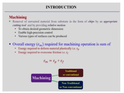
So machining at how, what is the purpose of machining in manufacturing processes. Normally, in machining process, we understand some removal of the material, so that we can get some desired shape and size and of course, that unwanted material that will try to subtract it from the basic material in the form of the chip and of course by using the appropriate cutting tool and definitely it is possible to remove the material.
