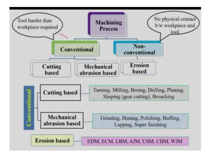
First, we the conventional machining process, what are the requirement? We need a tool actually the cutting tool to remove the material, but definitely when using the cutting tool that tool should be harder than as compared to the work piece material. So that is why some hardness difference must be there to remove the material and of course this is maybe more significant because there is change of the hardness with respect to temperature.
