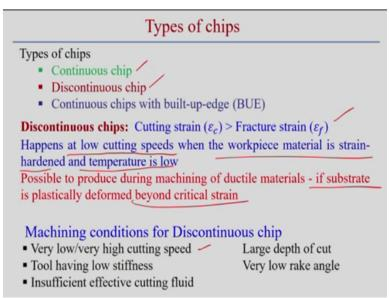
Now what are the different types of the chips normally formed in machining process. So types of chips, first is the continuous chip, discontinuous chip and the continuous chip with built-up edge. What are the different conditions to put different types of the chips? Discontinuous chips definitely discontinuous chips are produced, the chips actually breaks and there may not be continuous production of the chip. So theoretically chip breaks.
