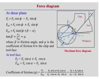
Now if you pass this surface force tag, we look into that. This is the tool a chip is flowing, this is the shear plane and we can draw. This is the resultant force R and we draw one circle, passes through the tool tip at this point. Now within that circle we can define the different force components and different angles also. So here this angle is shear angle. The shear angle can be defined such that the angle with respect to the shear plane and the cutting velocity vector with respect to that.
