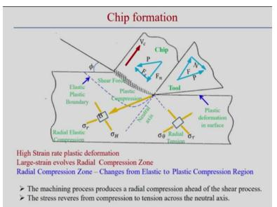
Now chip formation means, suppose this is a cutting tool. So relative motion between cutting tool and the work piece is moving these things, and then this cutting tool is cutting the work piece material and then it creates the chip and chip is actually by removing the extra material from the work piece in the formation of the chip and we can get that this is the machine surface. This is the typical elements of an orthogonal cutting process.
