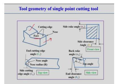
Now before doing that, we will try to look into the tool geometry of a single point cutting tool. In single point cutting tool, suppose this is the typical shape of a tool and of course it is 3 dimensional and if you look into different phase, different view, we can observe the different types of the angles, we measure to define the single point cutting tool. So of course single point cutting tool means the contact is in single point.
