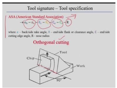
Of course, looking into this back rake angle and I think clearance angle and of course cutting edge angle, so then back rake angle, clearance angle, cutting edge angle, and of course nose radius, so this is called specifically the tool signature. There are 7 elements of tool signature, so 3 pairs of elements indicates three different types of the angles, rake angle, clearance angle, and cutting edge angle, and last one it indicates the nose radius.
