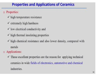
Properties and applications of ceramics I can see the properties it is a high temperature resistance that is the main properties and we can based on that several application is possible or ceramic components. Extremely high hardness, low electrical conductivity and therefore this can be used some insulating material, high chemical resistance as well as the lower density compared with the metals these are the typical advantages of the ceramics.
