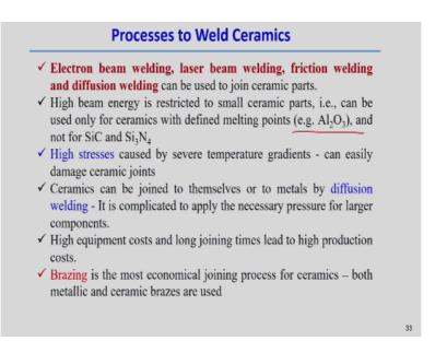
Processes to weld a joining of the ceramics is like that electron beam welding can be done, laser beam welding can be done, friction welding and diffusion welding normally all these processes are normally applied for the joining of the ceramic components. High beam energy is restricted to small ceramic parts for example can be used only for the ceramics with the different melting point.
