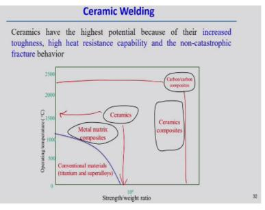
This is having the highest potential because of the increased toughness high heat resistant capabilities and of course and the non catastrophic failure fracture behavior. So therefore all these typical characteristics makes the (()) (07:46) of the ceramics is very difficult and most important thing is the ceramic is also very brittle if we look into that operating temperature and strength weight ratio.
