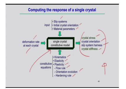
We can give an example also, for example computing the response of a single crystal structure. How we can do this things, what are the input required, if you see the input slip system, we should know for a particular metal what are the slip systems, then what is the initial crystal orientation and what are the material parameters is involved in this things and we should know deformation rate at each crystal what are the deformation rate.
