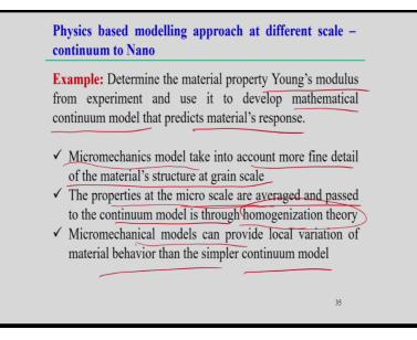
Now, we can give another example, for example determine the material properties Young's modulus, we know the Young's modulus we can easily measure in a particular material through experiments just by looking into the universal tensile testing machine for a particular material and therefore that value Young's modulus can be used some mathematical model in the continuum model, trying to develop the stress analysis for elastic stress for a particular material.
