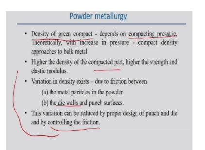
Then next step is that sintering process, but before that we can look into more on the compaction process. So of course the density of the green compact it depends on what pressure we are applying compacting pressure by the rigid tool and of course theoretically with increasing the pressure compact density approaches to the bulk metal in theoretically, but of course after compaction process it is sometimes it may not be possible to exactly achieve the density of the bulk metal.
