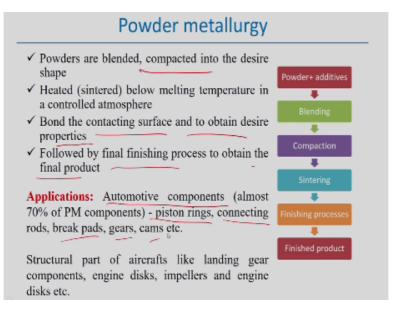
So powder metallurgy basically we understand from the terminology powder metallurgy that we made the compact product by using in the form of the powders. So the steps involved in powder metallurgy techniques if you look into this figure first preparation of the powders, making of the powders according to some desire size, shape and then we do some additives mixing or blending the powder along with the additives.
