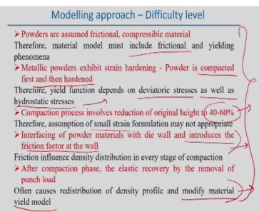
But before the approaches we can look into the in modeling of the powder metallurgy technique may be what are the difficultly levels we can look into that aspects first. So first point is that powders are assumed frictional and compressible material because we are compacting variation, so there is a powder initial volume (()) (36:47) accompany this is some kind of the voids between the powders when they are loosely packed.
