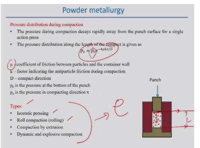
We can look into that the pressure distribution during the compaction process suppose this is the punch if you look into the this figure the powder particles are there. So definitely we can use the punch force here and such that powders can be compacted and they can rearrange among themselves we create the compacted with respect to each other of course it make some kind of voids maybe there in between.
