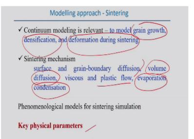
Now once compacting process is done then sintering process during this cases of course in the sintering process it is more relevant to consider the look into the grain growth, modeling of the grain growth densification normally happens because you predict the density of the product and the of course the deformation behavior during the sintering all this three are important aspect, physical aspects it is possible to model during the sintering process.
