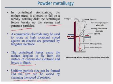
In centrifugal atomization the molten metal is actually allowed to fall on the rapidly rotating disk. So there is rotating disk and liquid molten metal actually fall on the that disk and then centrifugal force breaks the liquid metal up to the stream of the stream and that generates the particles actually. Now instead of directly looking to the molten of course there is one variation of this process use of the centrifugal forces here also.
