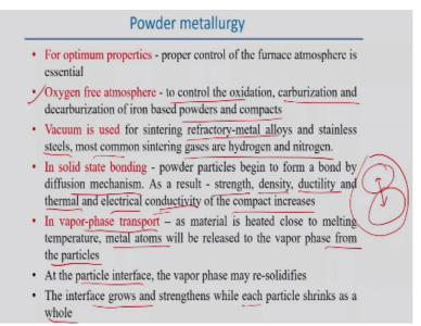
Now if we look into the powder metallurgy product so for optimum properties proper control of the furnace atmosphere is essential and of course controlling of the furnace atmosphere because it decides to optimum the powder metallurgy product then oxygen free atmosphere is mostly to control the oxidation, carburization, decarburization of the iron based powders and composites.
