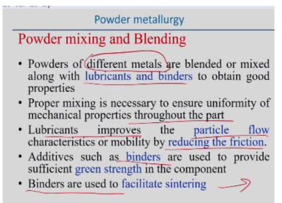
So once you produce the powders then we think about how to mixing and blending this powders. So powders of the different metals or similar kind of metals can be used are blended or mixed together and by using some lubricants and binders or additives to obtain good properties. Actually the lubricant and binders is normally mainly introduced along with the powder such that we can improve the properties of the powder metallurgy technique.
