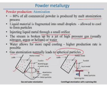
Now what are the different steps in powder metallurgy products. First is the atomization. Atomization melt, atomization we can say that means from the liquid molten metal we can produce the powder. So that is the most almost 80% of the commercially available powder is actually produced by the atomization process. So what is atomization process if we look into that and that liquid metal so directly liquid metal is fragmented to small particles, small droplets.
