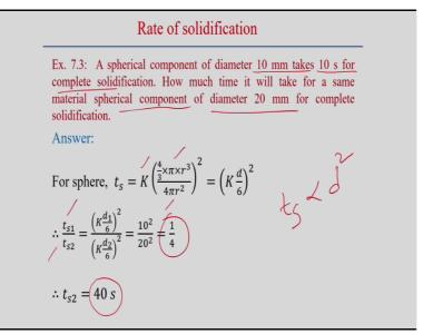
Another example you can look into that, we can look compare although same shape, spherical component diameter 10 second complete solidification but how much time it will take for a same material that means material is the same, same material spherical component of diameter that means sizes are different basically in this cases, one case diameter is 10 millimeter, another case diameter is 20 millimeter but they are having the shape is same, both are spherical in nature.
