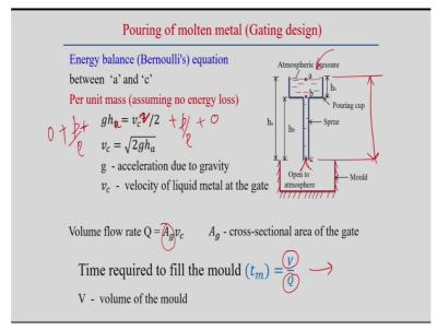
Now, we will try to look into this Bernoulli's equation in our problem, so for example here is a situation that pour the molten material on the reservoir but at the same time we need to maintain at the constant head that label of the point a is made as a constant and then liquid metal flow here and of course you see it is obvious that at point a also exist atmospheric pressure, at point c also atmospheric pressure.
