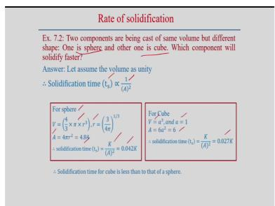
Now, we will try to look into that some simple problem to understand the rate of the solidification. So, for example two components are being cast of the same volume but different shape. Shapes are different, one is the sphere, other is the cube for example. Which component will solidify faster? Let us look into that. So, if we assume, volume are same, we assume the unit volume.
