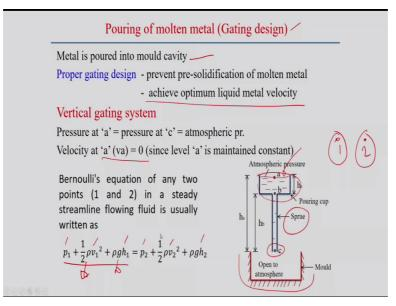
Now, next step is that after melting then we need to pour the molten material in the mould cavity but what we can these things that is better described by the is called the gating design. So, basically how to design the gate, gating system during the casting process, so the main purpose is that how the molten metal is poured into the mould cavity, (()) (10:48) if you see this specific schematic figure of this, so this is suppose this is the mould okay some this mould is open to atmosphere.
