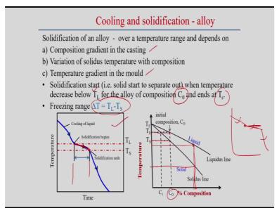
But we analyze this solidification process in case of for example alloy system because pure metal we have the melting point temperature, single melting point temperature but in case of alloy, solidification actually happens over a range of the temperature, normally in between the solidus and liquidus temperature. So, therefore this range of temperature actually depends on the composition gradient in the casting process.
