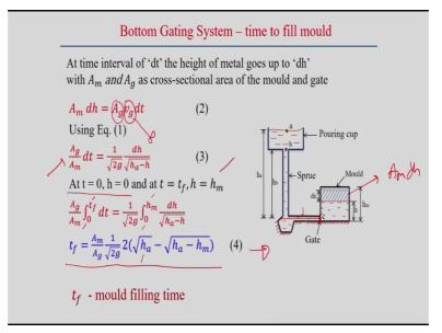
At that time, now we look into that elemental time dt and that elemental time dt, there is a increment of the height on the mould cavity that is dh. Now, we know that Am, Ag we defined the cross-sectional area of the mould as well as the gate, so maybe this was the runner, so at this point what is the cross-sectional area of the gate is I think we assumed as Ag. Now, we need to maintain the continuity equation here.
