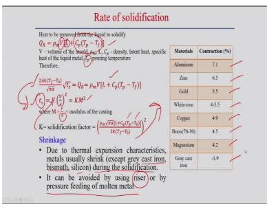
Now, what is the heat transfer to the mould material that is should be equal to what is the heat extracted from the liquid molten metal to solidify or to change the liquid metal to the solid metal. So, in that way other we can estimate what is the heat removed from the liquid metal that QR=rho m V is the volume of the mould and rho m Cp specific heat, latent heat all as the properties of the metal here.
