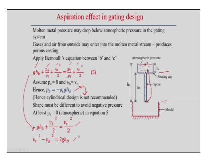
Now, if we look into that aspiration effect in gating design may be we estimated, assume the certain point the atmospheric pressure exist but if we look into very carefully the top gating system, the sprue within the sprue it is not necessary that atmospheric pressure exists. We can show simply by mathematical calculation also that there may be the variation of the pressure within this sprue and accordingly we need to design.
