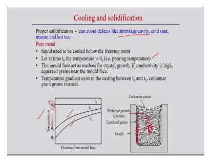
Now, we come to that point, the cooling and solidification relevant to the casting process. So, proper solidification is required or we need to understand how solidification happens basically what way the solidification is basically what way the heat is extracted during the casting process, accordingly you can avoid different kind of the defects. For example, proper solidification not done then shrinkage cavity, cold shut, misrun, hot tear.
