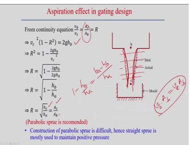
Now, from continuity equation that continuity equation that at this point between these two points b and c that velocity at vb\*the area Ab should be same as vc\*Ab. So, this continuity equation should be maintained. That means the volume flow rate at any section it should be
