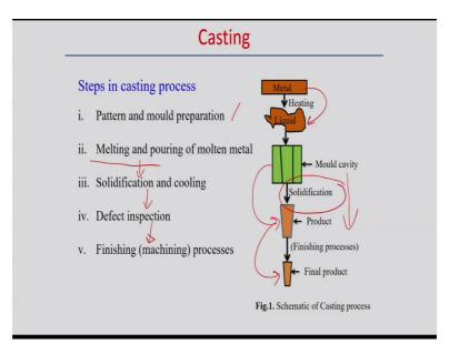
So, it is a well-known fact that casting process it is an almost standardized process but first we are looking into the casting process but specific to metallic materials. So, in first we need to melt the molten, we create the molten material and then the metal by heating and change the phase in the liquid phase and then that liquid molten material we then we put in the mould cavity so that mould cavity is the desired shape which we are looking for after solidification of a particular component.
