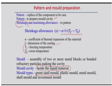
So, now first we look into that pattern and mould preparation and overall these things. So, pattern is basically the replica of the component to be cast. So, this has to be made according to the size, volume of the component we are looking for. So, this creates the cavity, mould cavity according to the shape of the pattern, shape and size of the pattern and that mould cavity actually filled by the molten material.
