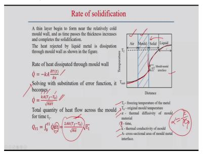
Now, we try to estimate the rate of the solidification during the process, we look into that in a particular process. Here we can see the air is there, then upon air is in contact with the mould material and then liquid metal certain part of the liquid metal solidify and this is the typical (()) (47:00) and temperature distribution is like that the liquid metal is above the melting point temperature within the solidified less than the melting point temperature.
