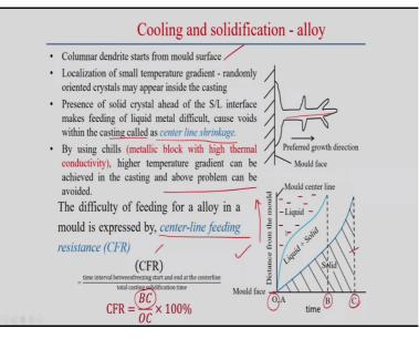
So, in general we can see that columnar dendritic actually starts from the mould interface and the dendritic form with the secondary and primary dendritic with that dendrite basically growth happens with the preferred growth direction and all depends on the temperature gradient in a particular direction. Of course, some sort of under cooling also responsible for the mode of the solidification but that is not our objective here.
