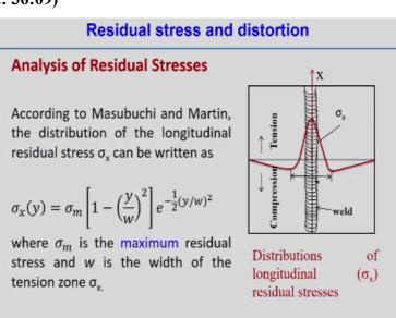
In general, you see the two longitudinal and transverse residual stress we can measure. Longitudinal means which direction the we can perform the welding process and suppose this is the longitudinal direction and we can say that this is the transverse direction. So this longitudinal direction, transverse direction, residual stress can also be measured experimentally.
