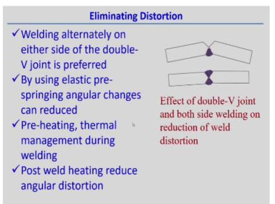
Other for example, in case of double-V joint, so one sided joint if you do it creates kind of distortion, but if you do the second joint also the distortion can be minimised and it can reduce the amount of the distortion when after during the second V weld. So basically welding alternately either side of the double V-joint is preferred, then why using the elastic pre-springing angular changes can be reduced.
