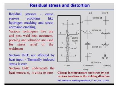
Now in welding process what we can explain the nature of the residual stress normally generate in any kind of fusion welding process. So here if you look into this figure that different sections suppose the welding has been done in particular directions and here we can see this is at any particular time this is the position of the heat source. Now if you look into the section A, already solidified, that means the temperature gradient is already 0.
