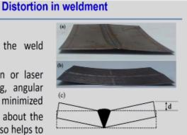
Distortion: (a) transverse and (b) welding direction (c) estimating the deflection in the butt joint Here we can see that very thin plate, but the other way also to reduce the distortion is simply by reducing the material volume. If we melt or this thing very small amount of the volume melting, by melting a small amount of the volume and that clears kind of the weld joint which is the 2 components that will also try to reduce the weld also.
