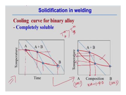
Now we will try to look into that how the just analyze of binary system that means assuming the alloy having the 2 components only say components A and components B and they are mixing this and they are making some kind of the alloy system of course the assumption is that they are completely soluble with respect to each other. So normally if we look into the time temperature diagram for an alloy system it is like that with respect to time.
