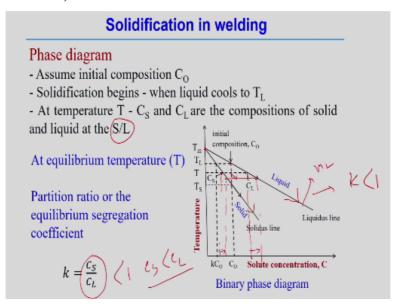
Now phase diagram so we assume the initial composition is the C0 particular position the solidification begins when we start at this point and ends at this point that there is a change of the phase at temperature T we see at a particular temperature T corresponds to this Cs is the and CL are the composition of the solid and liquid at the solid liquid interface. So SL means solid liquid interface.
