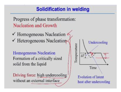
So progress of phase transformation nucleation and growth in general, but what are the different types of the nucleation actually happens during the solidification process. First one is the homogenous nucleation and normally we can say the heterogeneous nucleation, but what are the driving force for the homogenous nucleation and what maybe in case of heterogeneous nucleation.
