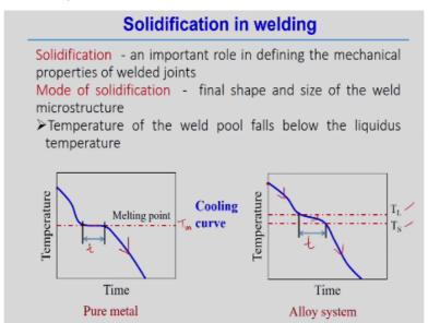
So first we try to understand how the time temperature diagram of a molten material looks like for example this if we look into this figure first figure. So this is the time temperature diagram specific for a pure metal. So you know it started with the super heated temperature and a very high temperature that means it is a liquid metal and then it comes to that at the melting point temperature.
