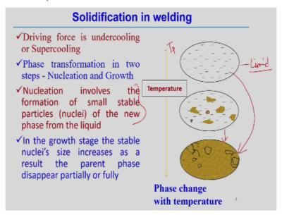
Now how solidification happens in this case if you see that in solidification that we start with the very that it is a initial phase it is a liquid phase. So suppose this is a peak temperature that very high temperature which is above the melting point temperature all metal maybe in the liquid phase and there is a decrement of the temperature. So certain point within the liquid phase there is a nucleation actually happens.
