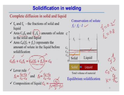
Now I will look into that complete diffusion in the solid and liquid we are assuming that this is a diffusion actually happens it is a solid and liquid diffusion in the solid and liquid phase such that we can estimate what is the solid fraction and liquid fraction in the solid the liquid fraction and solid fraction from the conservation of the solute. So we try to look into this try to look into this diagram.
