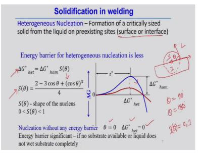
But similar kind of phenomena can be explained if we look into that heterogeneous nucleation process. So that starts with the formation of the critically size nucleus similar concept we can use here also, but heterogeneous nucleation start actually start over a surface or interface or in presence of any nucleating agents that sides or substrate actually to start to
