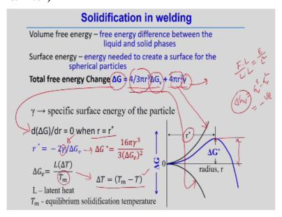
But to start the nucleation process we can look into that the volume free energy actually volume free energy is required to differentiate between the liquid and solid phase. So that normally we measure with respect to per unit volume and there is a surface energy changes which also required that is called the energy needed to create surface for kind of spherical
