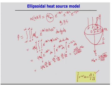
So, suppose the heat density distribution is something like that it is distributed over an ellipsoid and suppose this is axis x, y and suppose this is axis z and this define the ellipsoid, so further axis length say a, semi axis length along the x-axis is a, semi axis length along y-axis it is b and in z direction the semi axis length is suppose c and this of course this is the geometric shape of an ellipsoidal with the geometric parameters.
