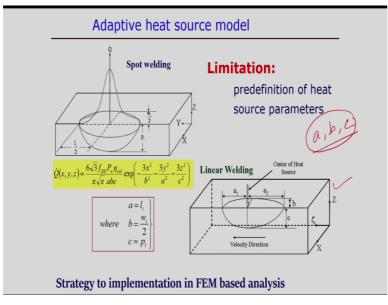
Now, we come to that point and the adaptive volumetric heat source model but of course before explaining these things what are the limitation of all what we discussed, double ellipsoidal or single ellipsoidal heat source model, the main limitation is that before start of the simulation, that means we need to define what is the value of all these geometric parameters A, B, C all these parameters we need to define.
