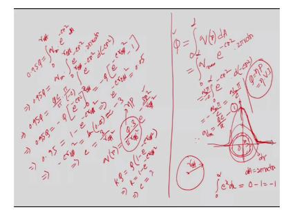
For example, if we see what is the total heat Q is exactly deposited on the workpiece surface that can be represented like that say q which is a function variable r and suppose over the elemental area dA. So, if we project like this suppose this is the circular area over which arc has been created and at the same time if we try to say the intensity distribution is the maximum at the center point and of course this is not exactly touch.
