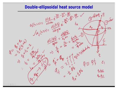
So for example heat source moving suppose x direction, so in this case this is ellipsoid 1 here the parameters are like that for example af is the semi axis length along x-axis and say suppose this is b and along the z-axis it is c for example and this is the other part remaining part, this another part of the ellipsoid which we merge this thing second ellipsoid, here also we having that this common parameter.
