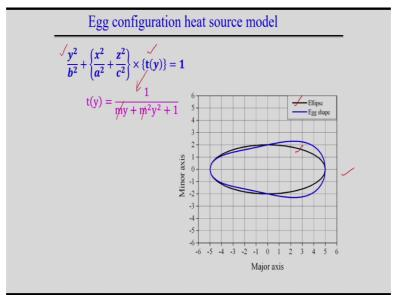
So, apart from the adaptive volumetric heat source, there is a development of the egg configuration heat source, the concept is like that we need to consider that ellipsoidal equation of the what the geometric shape of ellipse and but this term if you modify or introduce some functional form as a function of y, so if you see the y separate and here the functional form as y, then it actually modify the ellipsoidal equations.
