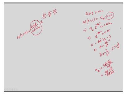
Now, distribution parameters can be estimated in other way also that if you see the intensity we represent in this way that this along x-axis is the boundary of the arc a, 0, 0 that means x, y, z; y=0, z=0 and x=a. The intensity is in terms of maximum intensity of only 5% of the maximum intensity that means 0.05. So, that means if we look into this expression that actually at the boundary the intensity is only 5% of the maximum intensity.
