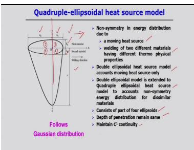
Now, we can shape in the continuation in the similar way, we can shape to the quadruple ellipsoidal heat source model but why it is applicable? So, like double ellipsoidal heat source model instead of taking two ellipsoidal merging in this cases in the four ellipsoidal we can merge and we can say this can be a quadruple ellipsoidal model but practically when it can be used, so this can be used in the specifically that welding of the two different types of materials.
