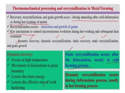
So of course recovery, recrystallization and grain growth normally happens during the annealing process. So annealing process is normally followed after the cold deformation or during the hot working of the metal. So this annealing after cold deformation or during the hot working of the metals so whether at low temperature or very high temperature all the cases it is a possibility of formation of the recovery recrystallization and grain growth during this process.
