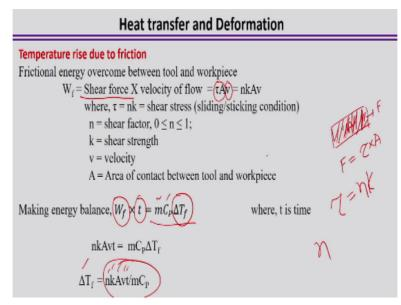
Now temperature rise due to the friction can also be estimated in the simplified way if we assume the frictional energy overcome between the tool and the workpiece. So therefore suppose this is the area (()) (09:48) friction is acting. Now that frictional energy can be estimated like that shear force because shear force and the frictional energy is basically the friction between these two surfaces.
