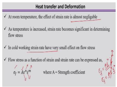
Now at room temperature we will see that what is the applicable normally at room temperature the effect of the strain rate is mostly almost negligible that means basically at cold deformation process the effect of the strain rate is negligible, but the effect of the strain hardening coefficients is more important during the cold deformation process, but once temperature increases then metals become softer.
