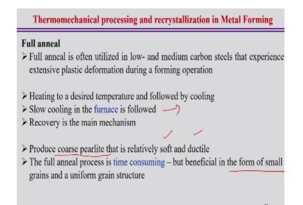
Now full annealing full annealing normally happens full annealing in the sense that when wide range of the carbon percentage exist within the steel so if you try to handle this kind of the steel through the heat treatment process we normally follow the full annealing process. So it is basically utilized for the low carbon as well as the medium carbon steel and that also experiences very high heavily plastically plastic deformation during a particular forming operation.
