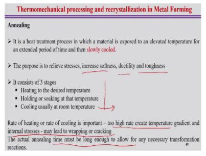
But before that what are the thermal process we normally follow that is more relevant to the metal forming processes first one is the annealing process because this is a very common process and it is a one kind of the heat treatment process that in the particular the metal is exposed at very high temperature and for a sufficient time extended period of time then you follow particular cooling rate.
