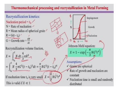
Now apart from the grain growth we try to look into the recrystallization kinetics and whatever way we can estimate roughly the recrystallization fraction. So the crystallization fraction can be estimated like that suppose this is the first we tried to look into the what is the recrystallized fraction. So suppose we have the sample and this sample having the old grain strain grain.
