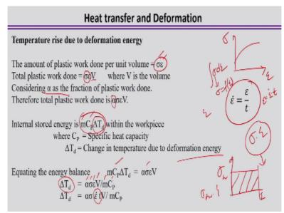
Now temperature rise due to the deformation energy. So we assume that there is a plastic deformation and we can simplify, but this simplified way we can estimate that. So the amount of plastic work done we can easily estimate per unit volume the simply stress and strain of course in this cases we are not assuming it is a simply multiplying by stress and strain, but we are assuming the average stress exist over the deformation period and over the deformation strain.
