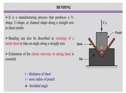
Apart from deep drawing process now I will try to discuss bending process in bending process what we can do in this cases we can get it from a flat sheet we can deform this in a particular shape and a particular angle for example we can produce the kind of v shape or u shape or maybe channel shape with respect to the straight with one straight axis in specific to the sheet metal.
