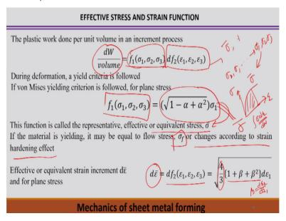
Now what is effective stress and strain function and effective stress and strain function is significant or important when we try to look into we try to represents the three-dimensional state of the stress. First if there is a three-dimensional stress states in a particular stress state. We can define in terms of the XYZ Cartesian coordinate system. There are 6 components sigma X, sigma Y, sigma Z, tau XY, tau YZ, and ZX.
