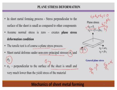
We can say the normally stress perpendicular to the surface of the sheet is small as compared to the other components and in that cases we can assume the stress is equal to 0 normal to this surfaces and that is called the plane stress deformation condition normally prevails in case of sheet metal forming processes.
