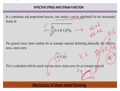
Now the effective stress value can be represented in actual true strain epsilon in instead of representing in terms of the incremental form because in case of continuous process or in any proportional process. So therefore incremental means it is a small now question is how small is this incremental strain? so therefore this incremental strain form can be is equal to epsilon. The epsilon 1 can be equal to epsilon one over a long range if process is continuous.
