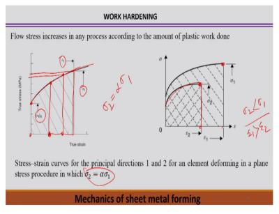
Now we try to explain the work-hardening. Of course we have some idea about the work-hardening and we have already explained what is work-hardening during the plastic deformation process. So we start with these things and we relate with respect to the flow stress because in sheet metal forming, the flow stress is more significant or important parameter. So therefore flow stress increases of course flow stress increases at any process according to the amount of the plastic work done.
