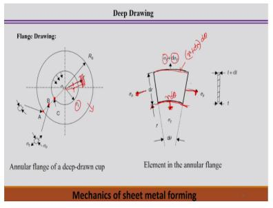
Now we look into the mechanics of this deep drawing process. So we consider the flange drawing process. So suppose this is the initial shape of the on a radially flat the flange having particular thickness and the punch the in that so the diameter ri is the punch within which there is a punch is acting there and then it is readily drawn to the depth, depth direction and outside up to from here to here it is a diameter R0 and that we define the 3 different points A,B and C.
