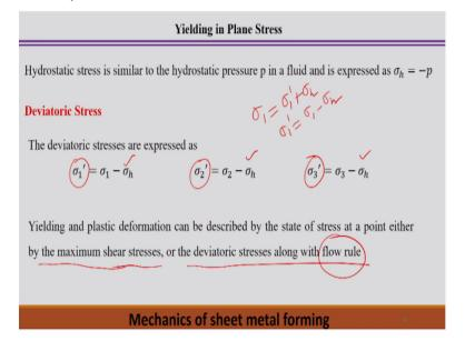
Therefore, hydrostatic stress is similar to the hydrostatic pressure that means p which is normally used in fluid mechanics and is expressed by sigma h=-p that means we change the sign because hydrostatic pressure in case of fluid mechanics it creates the compressive stress within that element. So that is why sigma h can be represent replaced by -p. There is another stress the deviatoric stress we have already talked about the deviatoric stress components.
