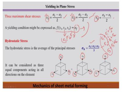
Which is expressed like this by this three equation. Now therefore it is possible to represent the yielding condition that means just start the yielding situation can be expressed as a function of this shear stress. So ultimately this shear stress is in terms of the sigma 1, sigma 2 and sigma 3. So it can be also a function of sigma 1, sigma 2 and sigma 3 and that is=the flow stress value.
