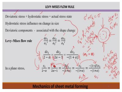
Now apart from this yield condition, the flow rule is some to explain the plastic behavior and when we try to explain the Levy Mises flow rule here we can see the deviatoric stress+hydrostatic stress that actually=the actual stress state. So similarly deviatoric stress sigma dot+hydrostatic stress sigma h=the actual stress. Now therefore hydrostatic stress influence on change in size.
