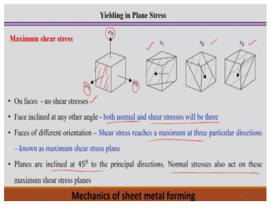
Now we try to understand the maximum shear stress and if we look into the a material point. In that particular material point, state of the stress maybe the stress tension sigma X, sigma Y, sigma Z and the shear stress component but we represent this normal stress and shear stress components in terms of the principal stresses. Such that this principal stresses sigma 1, sigma 2 and sigma 3 is acting of a particular element.
