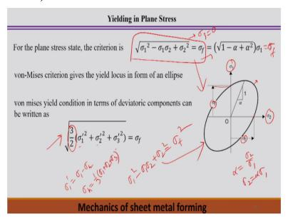
Now for plane stress the criteria can be here we can put simply sigma 3=0, the criteria Von Mises yield criteria can be modified that if putting sigma 3=0. Then it is become sigma 1 square-sigma 1 sigma 2+sigma 2 square=sigma f. This is the Von Mises yield criteria and this is corresponds to the plane stress condition. So now this can be expressed in terms of the stress ratio because alpha is basically sigma 2/sigma 1 or sigma 2=alpha sigma 1.
