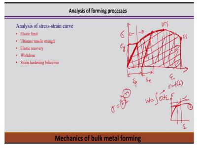
Now, before analysis of forming processes, so the analysis of the stress-strain curve is important in these cases. So, if we look into typical stress-strain curve for example in particular material metallic material it looks like elastic, so this is elastic part or we can say this is the yield point that yield point normally decides the transition from the elastic to plastic components.
