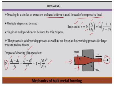
Similarly, in case of drawing process also, drawing is also similar kind of the extrusion process but tensile force is used instead of the compressive load. Here, we use the tensile load and instead of the compressive. Look into this figure, so in extrusion process, we used the compressive load but here in the drawing process, there is a thick diameter of that is very high and it is when we are given here the tensile load, so diameter is reduced from this big diameter to less diameter.
