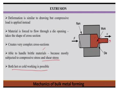
So, there are other metal forming process also that is called the extrusion process. So, extrusion process is simply there is a ram and the workpiece material. We just keep the compressive load by the ram to the workpiece material and this squeeze here and then it is the worked or deformed material actually comes out from this through this die. So, that is the basic mechanism of the extrusion process.
