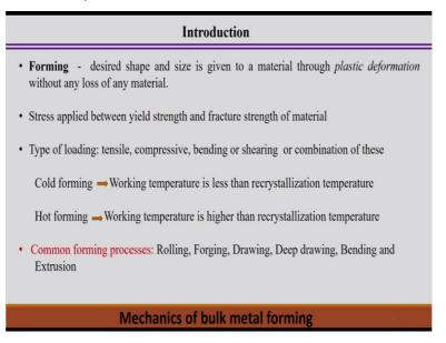
Forming, we get the desire shape and size is one kind of manufacturing process which is of course different therefore basic manufacturing process casting, machining, welding and one of them is the forming. So, we get the desired shape and size in the material and the material is normally so plastic deformation happens.
