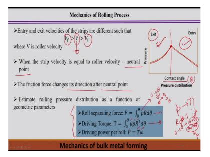
Now entry and exit velocities of the strips are different such that Vf is a final velocity or we can say the exit velocity and V is the velocity which is equivalent to the roller velocity. So, some point and Vi is the exit velocity. So, within this contact angle with that zone, the entry velocity and exit velocity are different and of course the exit velocity is less because there is a reduction of the thickness of the shape and entry velocity is more.
