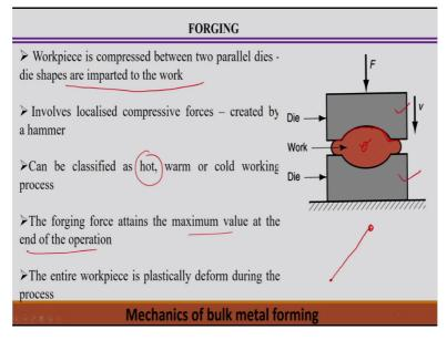
Now, coming to the next metal forming process that is called the forging process, say in forging process also similar phenomena in the sense that workpiece is there and we apply the force and of course workpiece is compressed basically between the two parallel die or maybe this is one die and this is another die and it can be with certain velocity.
