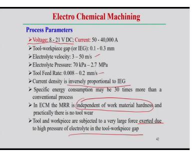
What are the process parameters normally followed here? In this case, that voltage normally 8 to 21 volt, if you see the voltage, normally DC current is used; current can be used from 5 to 40,000 ampere. Tool-workpiece gap or inter electrode gap can be 0.1 to 0.3 millimeter, so that gap is very small in these cases. Electrolyte velocity, basically high-velocity electrolyte can be passed through that gap.
