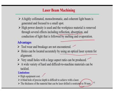
Say apart from this electro discharge machining process we can overall look into the laser beam machining process. So, laser beam principle is well known fact but in this case in laser beam that can also be used to several purposes laser. Well, laser beam machining also possible in this case, normally we use the very high power density laser to remove the material in this case.
