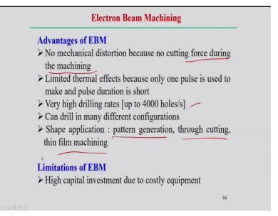
Advantages; mechanical distortion minimum, no cutting forces during this because it is also non-contact process, limited thermal effects and because in these cases not much time to thermal energy dissipated to the surfaces to the material. So, thermal the distortion is minimum in these cases, high velocity during, rate is very high in these cases, drilling different configuration more precisely.
