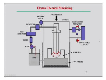
So, look into the schematically here, what is the electrochemical machining process, here this is the unit, so tool having certain shape and of course if you want to create that kind of the shape in the workpiece accordingly we need to choose the shape of the tool. So, then workpiece and such that uniform gap is maintained between the workpiece and the tool. So, similar shape of the tool we can replicate using this process.
