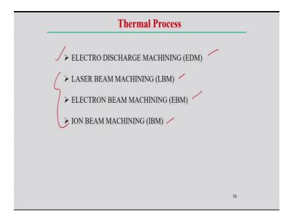
Now, if we look into the non-conventional machining process but under the category of the thermal processes, there are 4 different types of the processes; one is the electro discharge machining process, laser beam machining, electron beam machining and ion beam machining. These are the mainly 4 processes or maybe plasma machining process also exists that is under the category of the thermal processes.
