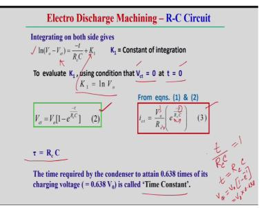
And from the integration, we can find out both the sides, we are going to find out this expression by integration. So, the K1 is a constant of the integration but K1 need to find out by using some kind of initial condition probably you can find out that at time t=0 basically
