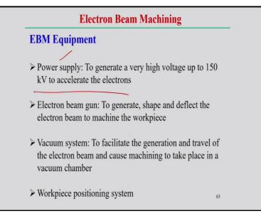
Now, electron beam machining process; similarly, we use the electron beam in this case instead of laser here and focused beam high velocity electrons actually impact on the surface can be drilling and machining, cutting operation can be performed using this process. So, very high velocity electrons basically strikes the workpiece, release the kinetic energy and converted to the heat necessary.
