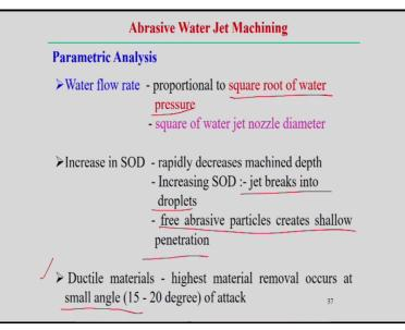
Water flow rate, parametric analysis can be done in that way that for example water flow rate, we need to maintain the water flow rate. It is basically proportional to the square root of the water pressure. It depends on square root of the water jet velocity nozzle. If you know the flow rate, water flow rate that means if there is increment of the pressure, the water flow rate will increase and at the same time if square of the water jet nozzle diameter.
