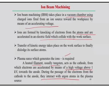
Similarly, ion beam machining process is simply takes place in the vacuum chamber but using the charged ions in these cases and of course we need a source of the ions and that ion source is deflected towards the workpiece where we need to remove the material and it should be accelerating, it should be accelerated in these cases. So, ions are formed by knocking the electrons from the atoms and are accelerated in the electric field which collides with the workpiece surfaces.
