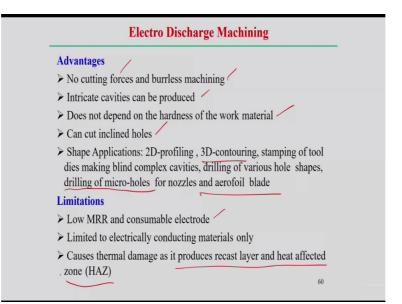
If you look overall what are the advantages and disadvantages of electro discharge machining process we can see no cutting forces and burrless, no cutting forces happens burrless machining process. Intricate cavities can be produced by this process, does not depend on the hardness of the workpiece material that is well known, can cut inclined holes also possible, depend shape application.
