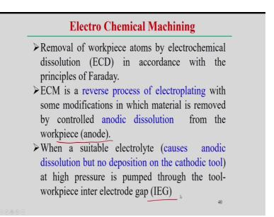
Here, the removal of the workpiece atoms by electrochemical dissolution normally happens in accordance following the Faraday's principle but it simply is a reverse process of the electroplating with some modification in which the material is removed by controlled anodic dissolution from the workpiece. So, workpiece is considered as an anode in this case and then how the workpiece or may be anodic materials dissolution happens.
