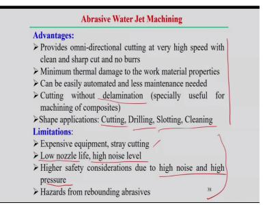
What are the advantage, disadvantage for abrasive water jet machining, you can see are listed here. If you see, it is a very cutting high speed with clean and sharp cutting and no bars can be produced using the abrasive water jet machining, minimum thermal damage because other way also when you sink the water is used, water is basically act as this heat sink in this case, so thermal damage can be minimized in abrasive water jet machining process.
