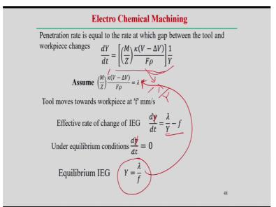
Now, if you replace J here, then we can find out the penetration rate is equal to the rate in which the gap between the tool and the workpiece. So, dY/dt we just simply replace the value of the J here. So, J here and we can find out that it can be expressed in this way the 1/Y and assume that this quantity is equal to lambda. So, tool moves towards the workpiece F millimeter per second for example.
