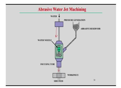
Here, we can see the schematic of the abrasive water jet machining process. So, water reservoir is there and then water comes from the reservoir and then there is a pressure generator through which the abrasive particles actually flows here and then water nozzle is here through once water comes out from the nozzles and then abrasive particles is added to the water nozzles and finally it comes out through this part and impact on the workpiece surfaces.
