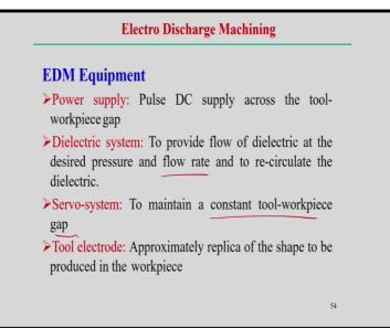
Equipment; simply power system is required power supply, DC power supply between the tool and the workpiece gap is required. Dielectric system is also required to control the flow of the dielectric fluid and basically to filter the dielectric fluid and with the maintain certain pressure to flow the dielectric fluid and of course pressure as well as the flow rate and of course recirculation is also then necessary in these cases is followed for the dielectric fluid.
