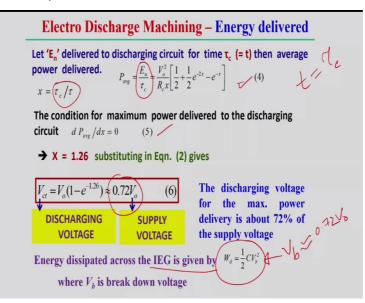
Now, let energy delivered to the discharging circuit for time tc, then average power delivered can also be estimated like that. So, suppose the En is the energy delivered to the discharging circuit but that En is the energy delivered to the discharging circuit for the time constant. So, here for example for the time so limit t correspond to the tau or we can say the time constant as a particular for a time tau c up to that time.
