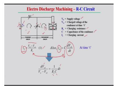
Now, we look into the RC circuit in the electro discharge machining process. We carefully look into that circuit diagram of electro discharge machining process, here we see that V0 is the input voltage supply here that the charging circuit and then in the charging circuit this is the charging circuit and this is the discharging circuit.
