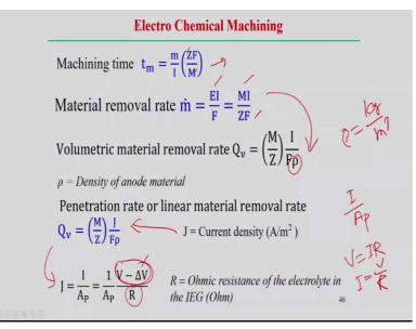
So, here we can estimate the machining time, this is the machining time can be like that if we go back to this formula that m this one, so here you can estimate the T=maybe mF/EI, such that similarly mF/EI, E can be represented Z/M. So, this is the machining time can be estimated here in this case. Then, material removal rate already estimated EI/F or MI/ZF, that we estimated the material removal rate in this process.
