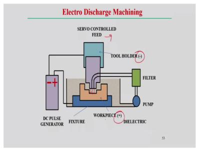
So, if you look into the unit that servo controlled feed system is basically to control the gap between the workpiece and the electrode and there is a dielectric fluid actually passes through that and of course dielectric fluid recirculate pumping, then filter and then that dielectric fluid again passes through the electrode and to the workpiece and then gap is maintained between the electrode and the workpiece.
