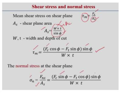
Now shear stress and normal stress during the machining process also we can estimate to prove you already estimated the shear force and then from here if you know from the Merchant's circle diagram, we know the shear force and from the shear force, we can estimate the mean shear stress on the shear plane. Here the mean shear stress on the shear plane, Fs/As. So Fs is the shear force acting on the shear plane.
