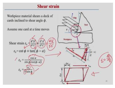
Now come to that point, the shear strength, but when we estimate the shear strength, here you can see the work piece material shears a deck of cards inclined to the shear angle phi. So we assume that a deck of cards which is equivalent to the formation of a chip and of course it is always questionable that up to what thickness you can know that means what should be the thickness of this deck. We assume some finite thickness deck.
