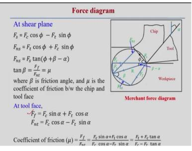
Here we can see that frictional force, which can be estimated in terms of these two components, cutting force components, one is that Fc which is parallel to that and normal to that force is the Ft. So Fc sin alpha + Ft cos alpha, in that form we can find out from this diagram. The frictional force and the normal force can also be estimated in terms of this Fc, Ft and along with the rake angle alpha.
