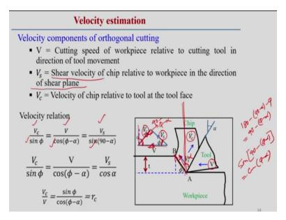
Of course if you look into the velocity, that what are the velocity components in the ideal orthogonal cutting situation, if you look into that process, two dimensional process the tool is moving with respect to velocity V. Of course, the chip also is flowing at a particular velocity, if we assume the velocity vector, which is parallel to the erect phase and that is called the chip velocity Vc and tool velocity with respect to opposite is V.
