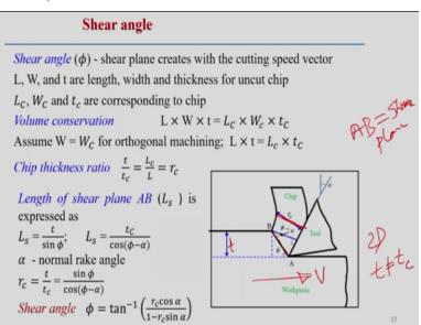
Now look into that what is shear angle here? Shear angle is basically the shear plane, if you schematically see these 2 dimensional figure, the shear angle can be defined that, so suppose there is a velocity of work piece relative in this direction V and then this is the shear angle, that basically this is the shear plane. Here you represent AB is the shear plane. So that plane making angle with respect to that velocity vector, that actually indicates the shear angle that is phi, well defined.
