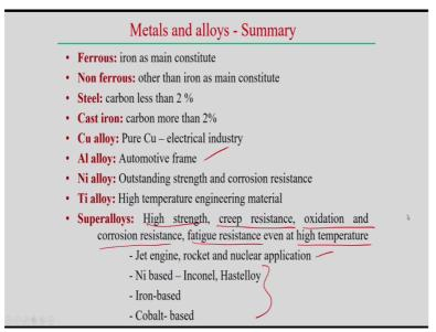
Metal in summary, metal and alloy we can see that ferrous metals we understand that iron is the main component, non-ferrous other than iron as the main constitute for the non-ferrous metals and alloys. Steels, we can categorize as less than 2% carbon. Cast iron, carbon percentage is more than 2% and then there are different non-ferrous alloy also, for example copper.
