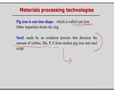
So, once pig iron is cast then once the pig iron is cast the desired shape which is called the cast iron and other impurities actually in the pig iron is forms into the shape through the casting process and that is called the cast iron and of course other impurities forms in the
