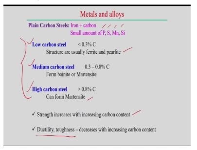
Now, this plain carbon steel may be the components of the plain carbon steel as simple iron+carbon but apart from that small amount of the phosphorus, sulfur, magnesium, manganese and silicon. So, these are the typical components of the plain carbon steel but we can see, we try to look into the overall look into that plain carbon steel can be different, three different.
