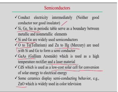
Then, semiconductor is the one type of the interesting properties of the one type of the materials, so semiconductors is basically conduct electricity between the metals and nonmetals, between the metals and insulator, so some intermediate way but in semiconductor the most important that what, the electrical conductivity can be controlled, that is the most important part in the semiconductor.
