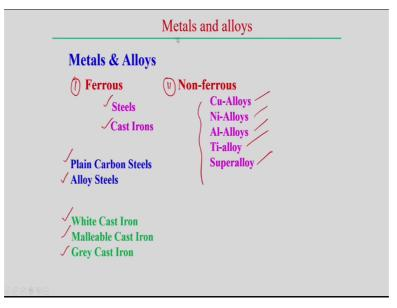
Then, if we categorize the different metals and alloys, we can see these are the engineering materials normally available. First is that metals and alloy we can categorize that ferrous metal two categories, first is the metals and alloys that in general ferrous metals and non-ferrous metals. So, in ferrous metals normally this steels and we can categorize the steels and cast irons and among the steels there are plain carbon steel or alloy steel.
