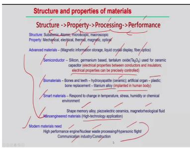
But we need to understand the properties of this engineering material and structure and properties of the engineering materials because the pillar of the manufacturing process and analysis is resting on the 4 steps. First one step the structure, property, how we can process and perform. First, if you want to understand the performance of a particular engineering component, then we need some relation and need to know what are the structure and the properties.
