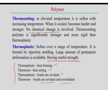
We can look thermosetting is basically at elevated temperature the material it becomes soften and then when it is cooled then we get the desired shape and it becomes more harder and stronger. So, therefore this process involves no change in the chemical composition and thermosetting polymer is significantly stronger, is more stronger, more rigid as compared to the thermoplastic.
