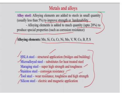
Now alloy steel, alloy steel apart from the not only the carbon is not only alloying elements but apart from carbon there are other alloying elements with small quantity normally added to improve or to get some certain type of the properties, normally the strength and hardenability and sometimes not only the strength and hardenability sometimes to impart particular for example if you want to impart the corrosion resistance, improve the corrosion resistance of a particular steel.
