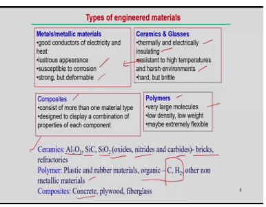
Now, with the introduction of the different manufacturing processes now we will try to look into the properties of the engineering materials or what types of the engineering materials normally used for the human being and for the development of the society. So, what are the different type of engineering materials normally is the 4 basic categories. We can see that first is the metals and metallic materials we can say.
