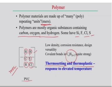
Now, we try to look into the polymer. So, polymer is, polymer material is actually made up of many poly repeating the mers units basically. So, one example, suppose this is one polymeric material, this is the one unit which is called mer, so repetition of the unit to form a long chain kind of things so that this is typical structure but polymers are mostly organic substances and containing the carbon and oxygen merely, carbon, oxygen and hydrogen.
