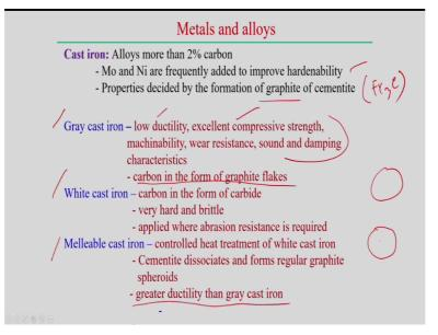
Now, we try to look into the cast iron also. Cast iron normally categorize when the iron along with the more than 2% of the carbon if we look into the iron carbon equilibrium diagram or phase diagram, we can see that more than 2% carbon is added with the iron that is under the category of the cast iron less than 2% it is under the category of the steel. So, apart from the carbon percentage in cast iron, there is molybdenum and nickel can also be added to improve the hardenability.
