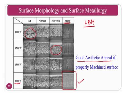
You can see here, some of the things you can do on your own, such as if you can control the atmospheric gases and other things, if you can control the various input parameters in laser beam machining. In the laser beam machining, if you can control the some of the input parameters like, laser power and the gas is that you are going to give. So, you can get very very good surfaces, in laser beam machining also ok.
