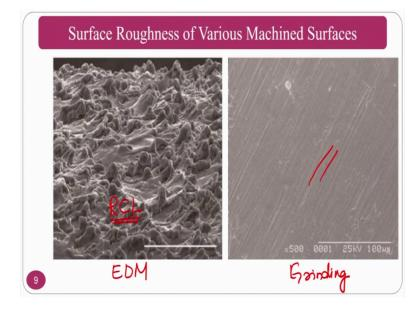
And you can see here EDM surface and at the same time a grind surface, this is the EDM surface are thermally destroyed surfaces and this is the grinding surface, or any abrasive process surface.
