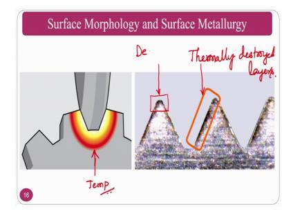
You can see here, whenever you make a some of the manufacturing processes, how the temperature destroys the manufacturing products? If at all I want to make a particular thread, in that circumstances because, of the form grinding or any other process are form electric discharge grinding process or this cannot be electric discharge grinding process because, there is a contact between work piece and tool.
