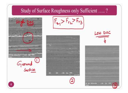
So; that means, the study of surface roughness is only important, you see the surface roughness of the ground surface, normally the grinding surface if you see here, these are the lay and you can see the plywood material and other things ok. This is grinding surface or ground surface.
