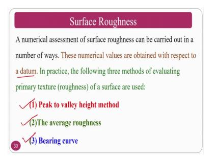
The surface roughness normally numerical assessment of the surface roughness can be carried out by number of ways; these numerical values are obtained with respect to the datum ok. In practice, normally the following methods are used. One is peak to valley height method, average roughness method and bearing curve, these are the 3 methods normally the surface can be measured or surface morphology can be expressed.
