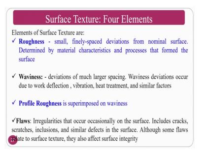
Surface texture you have 4 elements. One is a roughness, another one is waviness, profile roughness and flaws, that you have seen in the previous slides, you have surface roughness values, which is a high frequency low amplitude signals, waviness high amplitude and low frequency signals, if you are going to club both you are going to get a profile roughness, then flaws some of the metallurgical defects like, holes, ridges and other things.
