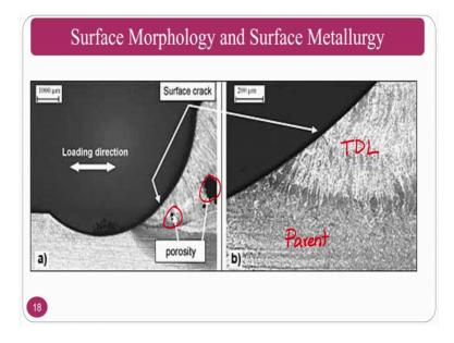
You can see here the metallurgical changes again, the porosity and other things are metallurgical changes porosity and other are whenever it is casted there may be a some changes, if you see the surface here, this is a parent material and this is the thermally destroyed layers or thermally deteriorated layers, these are the layers which are not to be manufactured.
