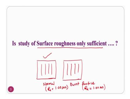
Is the study of surface roughness is only sufficient? That is the question. So, assume that I am going to get a micron surface roughness like, 1 micron. Is it sufficient? I mean to say is, if the surface is 1 micron, if it is metallurgically then there is no problem.
