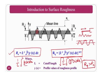
If you see this surface, where you can see the R a. R a normally is representing by the central line average value or a mean line and R q represent the RMS value, root mean square value ok. The equation is given and at the same time everything is given here. So, what is the physics or how the surface roughness can be measured? Whenever the probe moves on top of the surface, what will happen?
