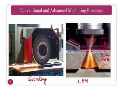
So, normally what are the advanced processes or conventional processes where you can see these type of thermal degraded layers is one is grinding process, that we have seen in the previous one, this is the grinding process, which can be called as a conventional abrasive finishing or machining process, another process where you will see the thermally degraded layers in advanced machining processes is laser beam machining process.
