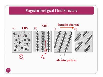
If you see the magnetorheological fluid structure as a CIP particles or the white ones, these are the CIP particles and the abrasive particles. So, how whenever the magnetic field is applied; that means, that H represents the magnetic field whenever the magnetic field is applied. This forms a chain and chain holds the abrasive particle, that is what the schematic diagram is shown here ok, that mean that when H is not there here and when the magnetic field is applied here H is applied.
