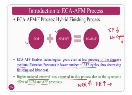
Electro chemical assisted abrasive flow machining process as I said this is the combination of electro chemical machining plus abrasive flow finishing operation, then it is called electro chemical abrasive flow machining or electro chemical abrasive flow finishing process. Electro chemical abrasive flow finishing process enables the goals even at low pressures of abrasive medium on less number of AFF cycles thus decreasing the finishing and labor cost.
