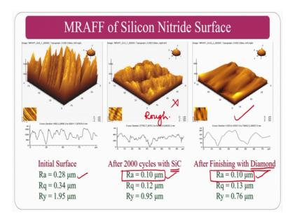
So, this is for silicon nitrate basically the work piece material is silicon nitrate. So, if you see the initial surface 0.28 micrometers 0.1 and 0.1 approximately with the diamond, but you can see the surface morphology, as I said their surface value may be looking same, but the thing that you have to see is how the surface morphology in the 3 dimensional look like.
