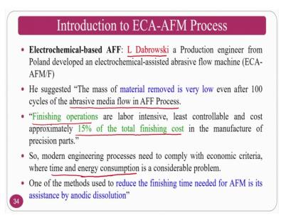
So, one of the methods to reduce the finishing time needed for abrasive flow finishing and it is assistance by anodic dissolution, one of the methods used to reduce the finishing time needed for abrasive flow finishing process and it is assistance by anodic dissolution process.
