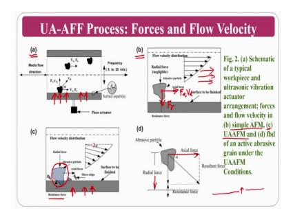
Now, we will see how the forces and the flow will takes place in the ultrasonic assisted abrasive flow finishing process. The first figure a represents the ultrasonic actuator assembly or connection to the normal work-piece in the abrasive flow finishing process and you can see here piezoelectric actuator is there which is connected to a couple and collate, where now you are going to give just vibrations to the work-piece.
