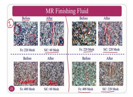
So, magnetic finishing fluid as you can see here before and after you can see the abrasive particles are randomly oriented and whenever you are going to apply the magnetic field. That means, that this is a before and after for the 60 mesh size of abrasive particle the chains are forming and this chains are held by the abrasive particles. You can see the abrasive particles are held, the similarly 220 mesh size iron particle are there and 220 mesh size silicon carbide is also there.
