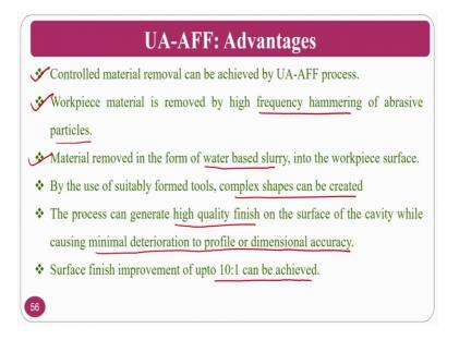
So, the advantages: the controlled material removal can be achieved by ultrasonic assisted abrasive flow finishing process, work-piece material removal by the high frequency hammering abrasive particles because of this high frequency dynamic motion what will happen, hammering will takes place and material removal will be increased.
