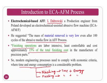
This particular process is the combination of electro chemical machining plus abrasive flow machining process or abrasive flow finishing process, as I said whenever I talk about abrasive flow machining or abrasive flow finishing process both are approximately same.
