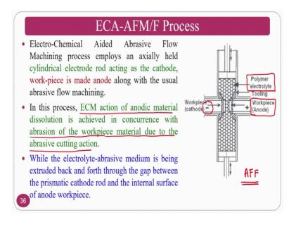
You can see here how the electrochemical process looks like, electrochemical aided abrasive flow finishing process employees an axially held cylindrical electrode rod acting as a cathode, work-piece is made as a anode which usually in the abrasive flow finishing process or abrasive flow machining process.
