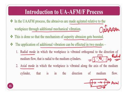
So, ultrasonic assistance abrasive flow finishing process abrasives are made agitated relative to the work-piece through the additional mechanical vibration; that means that the mechanical vibration is provided to the work-piece. This mechanical vibrations will try to agitate or try to make the work-piece into a dynamic one so, that the finishing action can be improved and material removal can be improved and the finishing time can be reduced.
