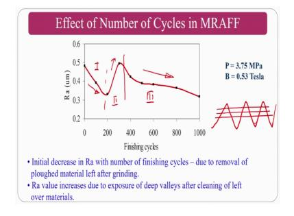
So, this is my surface and materials is here filled that is during the grinding process. So, initial cycles what is happening is here is it is shearing the surface because of which this region 1 I will divide into region 1, region 2 this is region 2, and this is region 3. So, region 1 what is happening is if you are sharing some of the peaks, what is the surface roughness is reducing that is what happening here.
