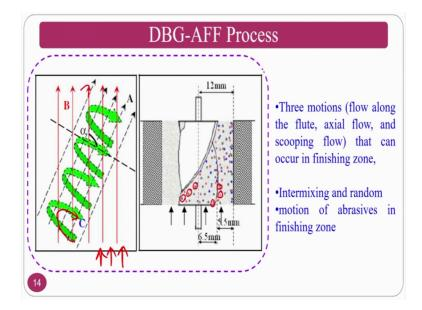
Now, we will see we have 3 motions; one is a reciprocation motion, and the second one is the along the flute direction motion, and the third one is scooping flow this green one is a scooping flow ok. So, the reciprocation shows the red colour one and the black colour arrow shows, the flow along the direction of the flute, and the green arrows shows the scooping flow.
