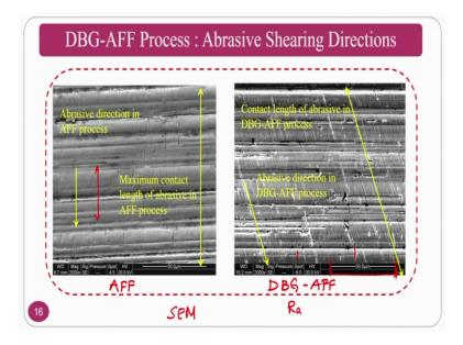
So, the radial force is high; obviously, your indentation will improve. So, you can see here in the abrasive flow finishing process and drill bit guided abrasive flow finishing process. In abrasive flow finishing process you normally see the minimum traverse length, because you are reciprocating. So, most of the time, it will be the shortest distance ok.
