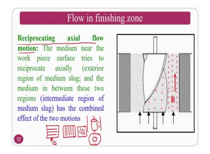
The second one is reciprocating axial motion; the medium near to the work piece. Because, this is slightly away from the flute and away from the drill bit in that circumstances. At the same time drill bit is a cylindrical surface, if you see my drill bit is a cylindrical surface and my work piece is like this ok. In that circumstances if you see the top view it will be like this.
