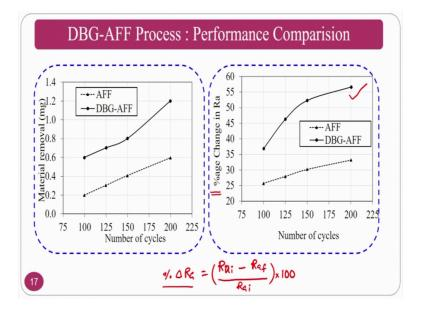
That you can see here the proper performance comparison of this process will with respect to abrasive flow finishing process. So, as the number of cycles versus material removal, if the number of cycles are going to increase; obviously, the abrasive particles that are cutting or the shearing the surface peaks will increase, number of times abrasive particles will cut increases; obviously, number of shear peak shearing also increases. So, the material removal will gradually increase.
