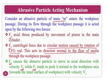
The considered abrasive particle with a mass "m" enters into the work piece. During the flow of through the work piece passage, F a is the axial force that is because of the medium reciprocation. I am explaining about the previous picture which you have seen. F c is nothing, but the centrifugal force due to circular motion caused by the rotation of centrifugal force assisted rod, which is normal to the flow of the medium.
