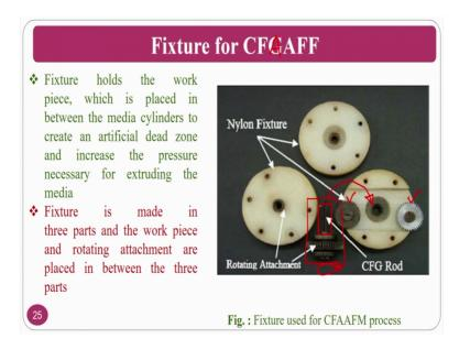
Now, we can see the fixture or the tooling for centrifugal force assisted abrasive flow finishing process. The fixture holds the work piece, which is in place between a medium cylinder and create the artificial dead zone and increases the pressure necessary to extrude ok.
