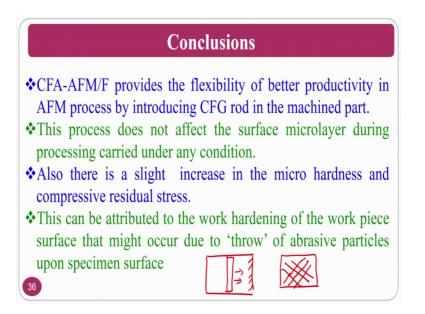
So, from these two we can see the centrifugal force assisted provides the flexibility and better productivity, and this process does not affect the surface micro layer; that means, metallurgical changes will not be there, and there is a slight increase in the micro hardness, and residual stresses also will be generated.
