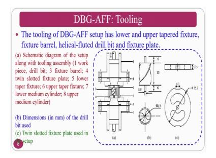
So, the tooling of Drill Bit Guided Abrasive Flow Finishing setup at a lower and upper medium cylinders and you can see here the same picture again it is there. So, these are the various elements are there; what you have to observe is how the medium is entering, how the medium is exiting.
