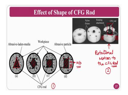
This is done and the shape of the rod. You can see here this is a nylon fixture that is what you have seen in a previous slide also. So, this is the rod centrifugal force assisted rod and which is get assistants from the other 2 gears gear 1 and gear 2, this will help to rotate at different speeds ok. So, the as I said the rotary motion will be provided from here, rotational motion to the CFG rod will be provided from here.
