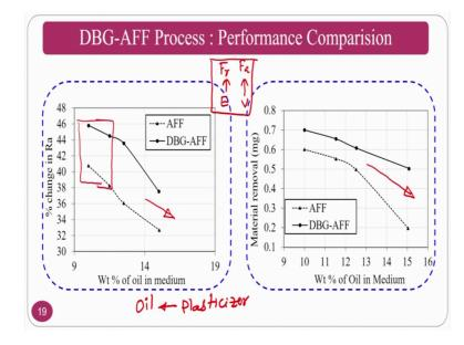
If, you see the weight percentage of oil; oil means plasticizer ok. So, you know in the abrasive flow finishing process what is the function of plasticizer and other things. Plasticizers are low molecular weight materials and polymers are high molecular weight materials, whenever you try to blend this, what will happen low molecular weight materials will go an sit between 2 polymer molecular chains and try to move apart.
