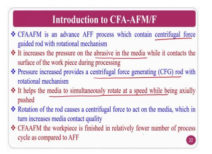
Introduction to centrifugal force assisted abrasive flow finishing process; just you have to get one correction here that is called CFA. So, centrifugal force assisted abrasive flow finishing process. So, introduction to centrifugal force assisted abrasive flow finishing process, it is an advancement of abrasive flow finishing process where centrifugal force guided rod will be there. So, they are going to place a rod with a different shapes and rotates at different speeds ok.
