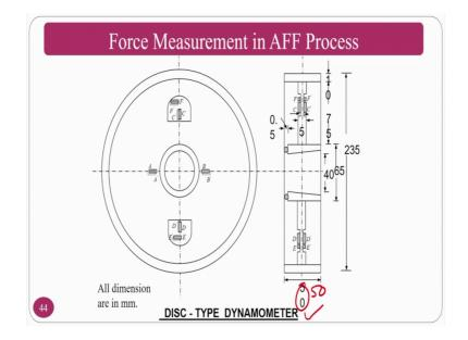
Once you have done this thing, then it is normally a disc type or ring type dynamometer that they have done. So, then now you have to balance the width stone beads and other things it is very common things that everybody will do. These are the dimensions of the disc type dynamometer, which is done at the IIT Kanpur. The schematic diagram, that they have done how they are mounting various sensors for measuring the axial force and radial forces.
