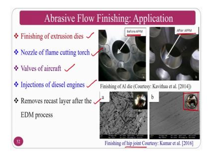
If you see the applications finishing of extrusion dies abrasive flow finishing process is required nozzle of the flame in the cutting torch, aircraft valves injections in the diesel engines, removes recast layer and other things these are the some of the applications where you are going to use ok. So, the dies industries you can clearly see the before abrasive flow finishing process and after abrasive flow finishing process.
