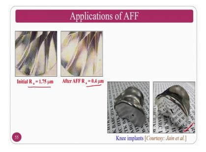
So, turbine blades (Refer Time: 40:15) turbine blades knee implants if you can see here initial surface is 1.75 microns and final roughness is 0.4 micrometres. The knee implant also this is another knee implant, you can do by abrasive flow finishing process, you can also do by the M R A F process and M R F process also ok. So, for a this process is done using M R F process. However, the same thing you can do by abrasive flow finishing process also.
