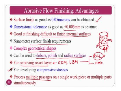
The advantages of abrasive flow finishing process the surface finish as good as 50 nanometres you can get, dimensional tolerances you can get up to 0.005 m m, and good finishing to difficult to internal surfaces, because internal surfaces some are some type of complex shapes will be there, sometimes there will be intersections will be there and other things.
