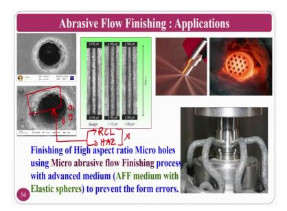
You can also do you finishing of this laser machine surfaces, because if you can see here this surfaces are thermally destroyed surfaces. This layers will have recast layers recast layer, heat effected zone, and many other zones. This recast layers has to be removed, otherwise whenever this come into practical applications these particles may go away and may causes lot of problem.
