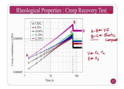
Now, we have to understand what is the viscous percentage, what is the elastic percentage in a medium. For that purpose we have to do the creep recovery test the creep recovery test. Means, you have to load or you have to strain the sample for a time and then you have to release. Now, it will undergo the viscoelastic change as well as elastic change the remaining will be viscous.
