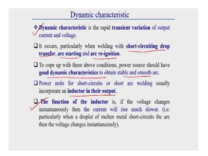
Now, we will go to dynamic characteristics of power source. So, we already discussed in details about the static characteristics of power sources now we will go what are the dynamic characteristics of power source. In case of a static characteristic power source the output is not tangent it generally there are tangent variation or generally there is not rapid change of current and voltage is not there or generally this output it is not depends on time.
