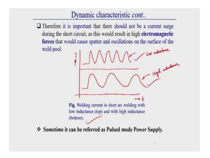
Now, here generally I am just showing then I will what is the function of inductor with output current or voltage output current. Here I am just showing a figure then you will get a very good idea from here. Let this is time t; this is time t here generally I am showing two figure here generally. Here this axis represent let us current I. So, how the current is varying?
