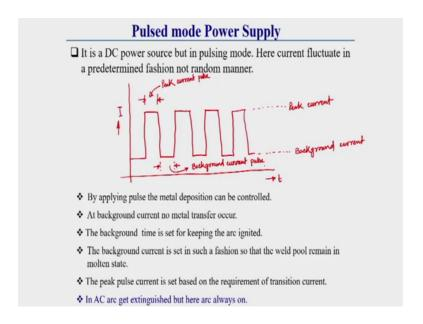
Now, what is pulse mode power supply? Pulse mode in pulse mode power supply also is a DC direct current power source, but here the output is pulsing mode. This is also direct current power source, but it is output is in pulse mode, this pulsing or; that means, this rate of change of current or voltage which is not arbitrary here generally this pulse mode is predetermined; that means, what should be the number of pulse that is predetermined here it this pulsing is not come arbitrary.
