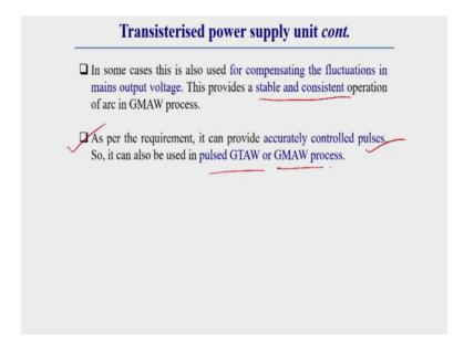
Apart from this thing in some cases this transistor power supply unit also can reduce the fluctuation in main output voltage; that means, it can compensate the fluctuation in main output voltage also. That is why, by this power supply generally we can get a stable and consistent operation of arc. So, by this we can get a stable and consistent operation of arc or this provide a stable and consistent operation of arc especially in GMAW process.
