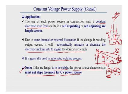
Now, for these characteristics; that means, for this characteristics this constant voltage power supply characters for power supply have some a special name. What is this a special name, that I will tell. Now, you see here one things you can observe, the application of this power supply, generally used where there is a constant feed of filler wire is there. That means, especially this is used for automatic types of welding.
