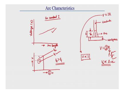
What is the characteristics of a arc? Generally arc means once we go for doing welding then generally in between the gap there is generally developed a arc this is generally called arc. So, what is the; what is the characteristics of arc? Which is very much important before going to detail about characteristics of power source. So, these arc means here in between this work piece an electrode this is actually electrode and this is actually work piece.
