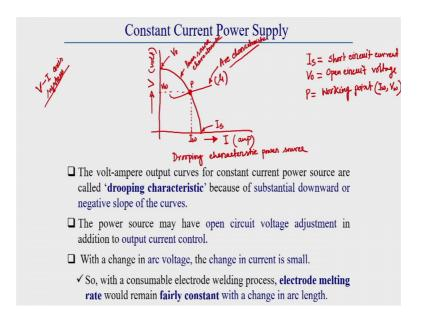
Now, we will go one by one about this is static power sources characteristics in details. So, first of all we will see, what is constant current, power supply characteristics? Generally constant current power supply characteristics curve, we can represented in terms of generally all the characteristics curve is represented in V I axis system V I axis system; that means, voltage ampere axis system generally, all the character generally
