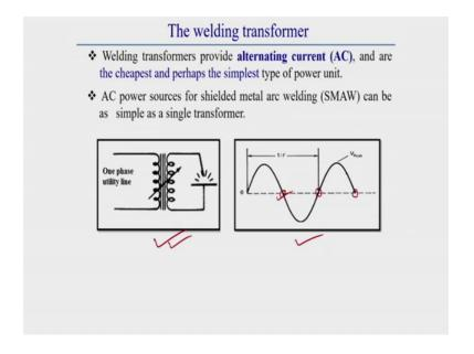
Now, we will see what are the different types of AC power source. Generally we have seen generally this simple AC power source is a simple transformer. This simple transformer generally used for SMAW and this output is what I have already this is a sine types of curve is there. Here we have seen there is every cycle there is a zero crossing is there ok; every cycle there is zero crossing.
