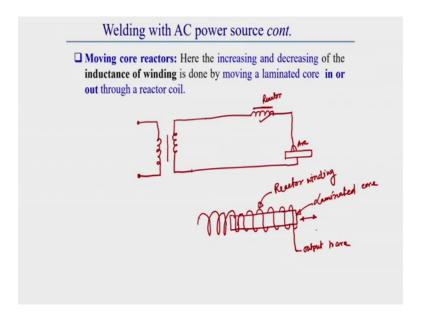
So, in moving core reactor generally which is similar to this power unit moving core reactor is similar to; that means, circuit is similar to that tapped reactor except that here is a moving core is there, here there is a moving core. This reactor is this is generally this reactor is generally here is a reactor which has a moving core that I will that I will show now. So, how its look like, what is moving core look like. So, this is here generally it is connected to the arc.
