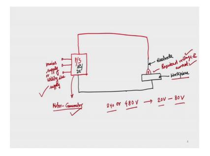
So, we got a idea generally to do the welding, what is required? A power source is required; a power source is required; let this is the power source. Why this power source is required? Generally by this power source only the by this power source only we can generate a arc, by this power source only we can generate a arc, we can generate a arc which is suitable then, we can generate a arc, we can generate a arc in between the work piece and electrode, in between the workpiece and electrode.
