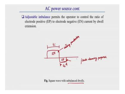
In case of unbalanced dwell power source, generally it is generate a dwell period its generally generate a waveform which have a which have generally 2 different dwell. Let this is t i and let this is t ii. Always keep it in mind that here which one is positive and which one is negative in this wave form. Always keep it in mind, this is generally
