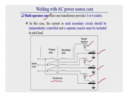
Multi operator sets power source means this types of transformer generally can provide 3 or 6 outlet at a time; that means, from a single transformer from a single transformer, we can get either 3 outlet or 6 outlet at a time.
