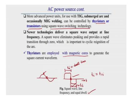
Now, next generally some other types of sorry generally this 3 different rectifier control reactor control 3 different reactor control. Power source we have seen. Nowadays generally also we get some other advanced types of AC power source. This AC power source generally is controlled by either thyristor or transistor.
