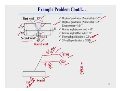
Now, we will see a example of this multiple reference line and what will be the welding symbol for a multiple operation of a multiple operation of a welding proce[ss]- ah. What should be the welding symbol for a multiple operation. Let us this is a geometry of multiple welding operation here let us here on si[de]- top side generally we did some welding operation which have different joint geometry and bottom side also we did some operation which have some other joint geometry.
