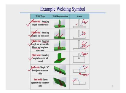
Now, we will do some example actually once we do some example of this weld joint then it will be very clear to us. Let us this is a welding operation that then first case here generally let us in a T joint we did a fillet welding whose leg length is 6; that means, 6 millimetre leg length lets. So, let us here this side I am interested to put the welding symbol. So, if this side we will put the welding symbol then what will be the welding symbol here.
