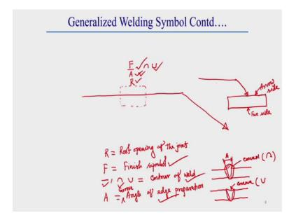
Here let us let this is a welding symbol, this is a reference line in this middle region. In this middle region general all the specification or all the details of joint geometry is provided. Like generally here generally it is represent you can say it is represented like this F A and R and after this F there is generally used a line for this line can be other type also that I will show in details. Here F A R is provided, what is F represent?
