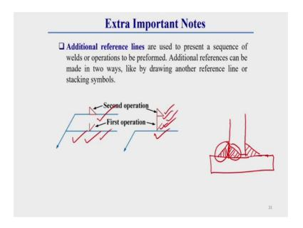
Now, this is the last part of this weld symbol that where here generally some sort of cases I have already explained in detail about different welding sequence if we perform in same side of a welding joint then what should be the different operation. Let us for a
