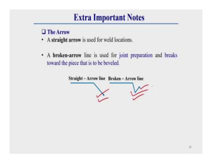
Now some other extra information we should know about welding symbol like in case of weld symbol there we will see two different types of reference line. Generally used one reference line is a straight another reference line generally broken types of reference line is used. A straight line generally used in welding this is generally this a straight arrow was once there is a straight arrow then this is used generally in direct field in the field of welding operation.
