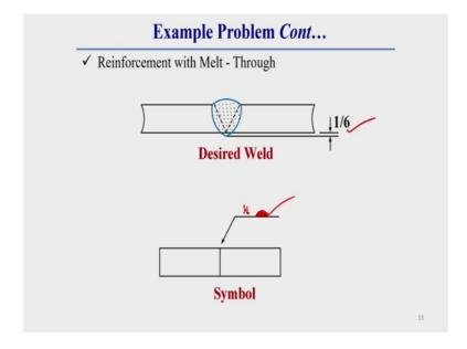
Now, we will see this already I have told you generally reinforcement and melt through is represented the generally in other side of the weld symbol which is look like this. This already I have which is look like convex shapes field convex shape. And this size of this melt through generally represented size of the melt through should represent left side of the left side of the weld symbol. That means melt through symbol here 1 by 6 we have to put left side of this melt through symbol.
