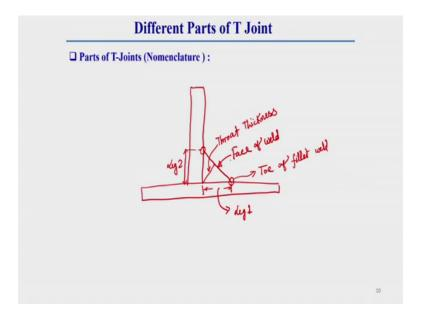
Now, we will see what is the different part of a T joint also. That way that means, in case of a T joint what are the if we do the welding then what are the different part of part are there. In case of a T joint the different part of different name also; like this let this is a inverted T here once we do the weld welding then this T this shape of the welds trianguler in nature which I have already discussed in detail.
