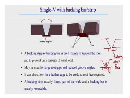
Now, here another extra information which is very much essential to know that is generally backing bar or backing strip. We should know what is backing bar or backing strip generally a backing bar or a baking stiff is used mainly to support the root. Generally in this root I have you know about every element of a welded joint. So, here the root is this thing generally to support this root this backing bar or backing strip is used backing bar or backing strip is used strip or bar is used.
