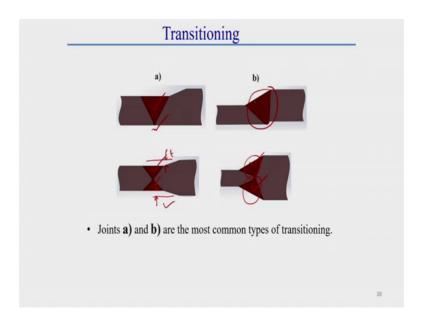
This is generally a common types of transitioning like this transitioning can be done like this here first of all is done after that here then only welding is done this transitioning can be one side this transition and can be both sides also. Here you see these sides generally thickness reduction we do thickness reduction is required to do. And similarly this side also thickness reduction is required to do this side let this is.
