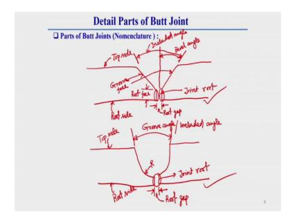
So, now we will go to the another element of the. So, now, we have already discussed about different part of a weld joint. Now we will see in a in a single in single butt joint what if the different part of weld joint in all the all the joint element now I will show in a single joint. Like let this is a butt joint here I will show you in detail about all the element of a butt joint.
