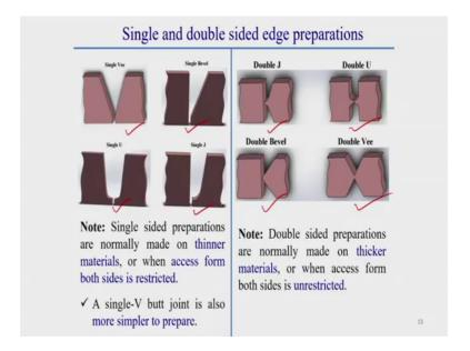
Now, these are also some extra information which is very much essential for welding purpose. Like single and double sided edge preparation. Generally; the single sided edge preparation one the edge preparation is done one side only. And this is the double sided edge preparation which generally required to prepare in both side of the weld joint. Now where the single side welding is required to apply and where this double side welding is required to apply that we should know.
