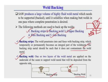
Now, as the submerged arc welding process is a high deposition what I have already told you high deposition welding process and what happens in this welding process generally we can get a large volume of highly fluid weld metal. So, what happens once we go for using this welding process for single pass butt welding process then to support this high fluid molten weld metal to drop out from backside of the welding welded joint generally there is used some baking to support that molten weld metal.
