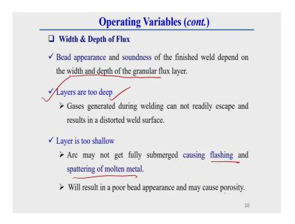
Now, width and depth of flux. This is a very essential or important parameter in case of this submerged arc welding process generally bead appearance and soundness of finished weld they depends on the width and depth of the granular flux layer. So, width and depth of granular flux layer provide the bead appearance as well as soundness of the welded joint.
