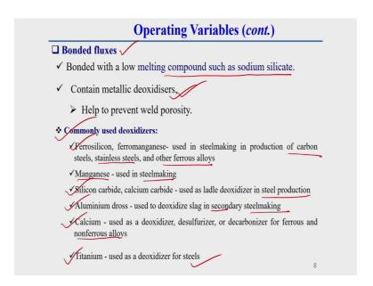
So, first of all bonded flux here it is called bonded flux because generally this granular fusible flux which contains some bonded element; that means, this granular fusible flux generally bonded with some low melting compound such as sodium silicate. So, whatever the flux composition I have told you in previous slide with this there is use
