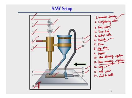
Now, this is the complete setup of this submerged arc welding process. Here one by one I will explain in detail this first one is called consumable electrode. It is called generally consumable electrode this one this one by one I will explain here what are the different part of submerged arc welding setup. The second one is called straightening roller.
