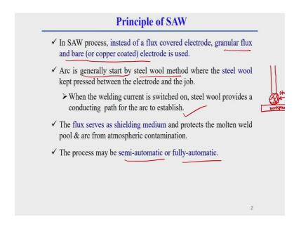
This is the principle of this submerged of this welding process. In this submerged arc welding process generally what I have already told instead of a flux covered electrode whatever used in SMAW process here generally granulated flux and a bare electrode is used then like in SMAW process there was used a flux cover and what happens flux covered electrode here generally a bare electrode with flux generally here is used.
