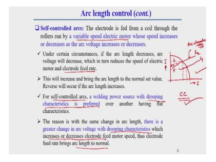
Now, in case of self controlled arc in case of self controlled arc here generally the electrode is feed from a coil through the roller which is run by variable speed here one things you should keep it in mind here variable speed electric motor is used, whose speed increases or decreases as the arc voltage increases or decreases.
