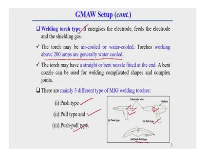
Now, we will go to the details what is this gun whatever gun or torch we have seen this torch have different types actually. This torch is the main part of this welding process because what happens it energize the electrode, feed the electrode and it also supply shielding gas to weld pool that is why this torch is very important part of this welding process.
