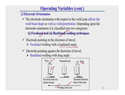
Now, now another important parameter is called electrode orientation this is a very interesting parameter electrode orientation with respect to actually weld joint affects the weld bead shape as well as weld penetration. Depending upon this electrode orientation
