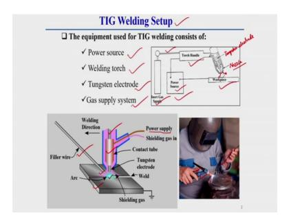
Now, this is the TIG welding setup or we can say GTAW welding set up here the equipment used for TIG welding here it is showing, here use a inert gas supply cylinder, it can be argon gas, it can be helium gas or it can be a mixture of argon helium gas. Here is used a power source this is the power source with this inert gas holes is connected to this torch and it is go to this nozzle here you see this is called nozzle and this is called tungsten electrode tungsten electrode.
