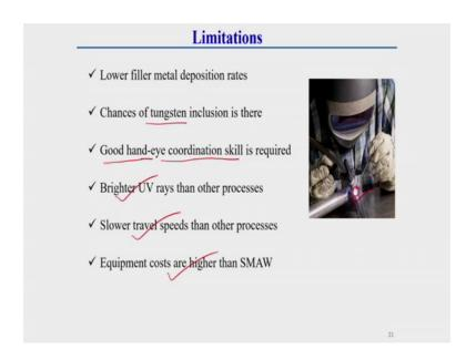
Now what is the drawback of this limitation of this welding process? Here one things you keep it in mind here generally lower filler material deposition rate comparatively lower than mig welding process. Generally here metal deposition is less and just here is used tungsten electrode so there is a chance of this tungsten melt and deposited towards the molten metal.
