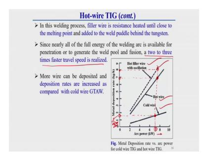
So, what happens here you can say that whatever the arc force or arc energy is that that generally directly supply to the molten pool. So, here generally more forceful arc and more forceful arc we can get. So, what happens due to these things, by this welding process generally we can increase deposition rate as well as penetration. So, what happens for this reason this welding process or this techniques can be two to three times faster than the cold wire TIG welding process.
