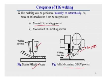
Now, this is the categories of TIG welding process, now we will discuss what are the different categories of TIG welding process. Generally this TIG welding can be done manually or it can be mechanised also, that is why depending upon this mechanism it can be categorize in two different categories one is call manual TIG welding process manual TIG welding what I have already discussed during categories of different welding process.
