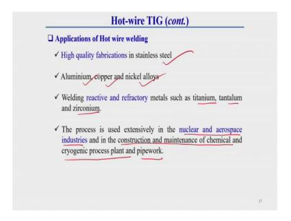
Now, this hot wire TIG welding techniques have huge application is has in early application it is its apply in high quality fabrication lie in stainless steel it is used in
