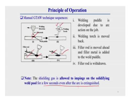
Now, will go for what are the different sequence of this welding process that also we should know because how the welding is start and how it should finish and what should be the sequences of this process that is also you should know that I am showing here.
