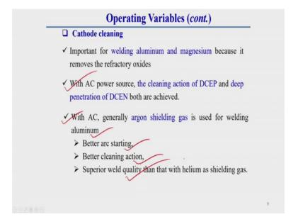
Now, here cathodic cleaning action I will discuss here in details, generally here a cathodic cleaning action is taken place with alternating power source and here one thing you keep it in mind with AC argon shielding gas is used for welding aluminum or magnesium; because once we use AC current towards there, then and argon gas is there then there will be better arc starting, better cleaning action and superior weld quality.
