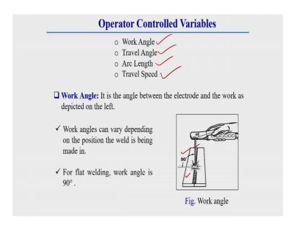
Now, here generally so these all about the different constituents of welding process. So, now we will go for what are the operator controlled variable. What are the different types of variable which can be controlled by a operator here? Actually I am not discussing about what are different operating variable of different welding process because what
