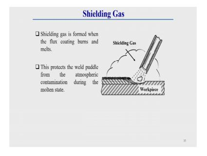
Now, the other constituents is shielding gas. What I have already told you shielding gas is generated due to the burning of the flux cover. That means, once this flux cover burned, generally it produced some gases. This gases generally protect the molten pool or we can say molten puddle from atmospheric contamination. So, that is why its act as a shielding medium that is shielding gas actually.
