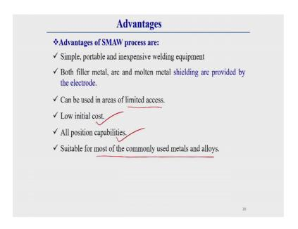
Now, we will discuss that what is the advantage of this welding operation? What is the drawback of this welding operation? Then what is the application of this welding operation in details. Here you see this welding generally have different advantages these are the following advantages we can observe in this welding operation like first of all this
