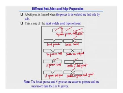
Like different butt joint with their edge preparation, you see by applying generally different edge preparation in butt joint, there can be different types of Bart butt welding joint. Like, you see here generally the edge preparation is done, here generally the edge preparation is done, in first categories a square type edge preparation is done. That is why in this welding process known as a square groove butt joint.
