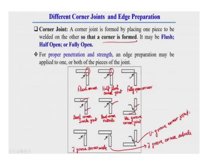
Now, different types of corner joint and their edge preparation, this corner joint also can be the corner joint we can define a corner joint is formed by placing one piece to be welded on the other. So, that a corner is formed here you see. So, that a corner is formed. It may be flush half open or fully open categories.
