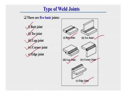
Generally, there are 5 different types of welding joints are there, where these 5 different welding joints are one is called butt joint, another one is called tee joint, another one is called lap joint, another one is called corner joint, and another one is called edge joint. This symmetric diagram shows this is first one is butt joint, this second one is tee joint, third one is lap joint, corner joint and edge joint.
