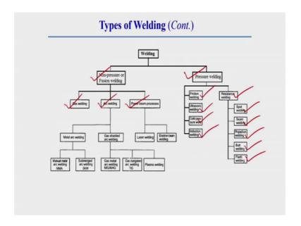
So, depending upon the pressure application of pressure the welding can be categorized into non pressure welding, or fusion welding or it can be pressure welding.
