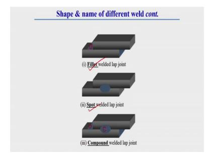
Now, here you see these are the different shape of lap joint. Here, you see here generally fillet welding is done, this is a fillet welding is done, that is why this is called fillet welded lap joint. Here, generally a spot welding is done that is why is called the spot welded lap joint. Here both fillet as well as a spot welding is done, here you see this triangular shape weld as well as this spot weld shape also we made, that is why this is called compound welded lap joint.
