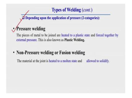
Like depending upon the application of pressure, this welding can be further categorized into 2 different categories. This can be on a pressure welding, another categories can be non-pressure welding or this is sometimes called fusion welding, this is popularly known as fusion welding.
