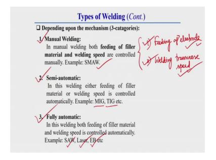
Now, depending upon the mechanism this welding can be categorized into another 3 different categories or 3 different categories, this can be manual welding, this can be semi-automatic welding, or this can be fully automatic welding.
