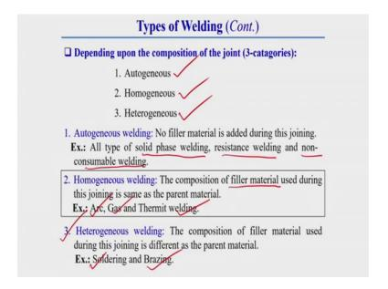
Now, depending upon the composition of joint this welding can be further categorized into 3 different categories; it can be autogeneous, it can be homogeneous, or it can be heterogeneous.
