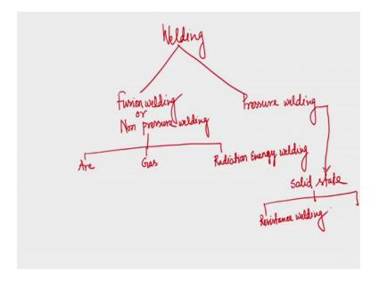
Depending upon this application of pressure welding can be categorize into 2 different categories; one is fusion welding, one is fusion welding, another one is pressure welding. This fusion welding is also is, this is also called fusion welding or non-pressure welding.
