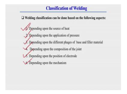
Classification of welding actually I have already started in yesterday's class, where we have seen there is different aspects based on different aspect, we can categorize the welding process in 6 different categories. That can be depending upon the source of heat, depending upon the application of pressure, depending upon the different phases of base and filler material, depending upon the composition of the joint, depending upon the position of electrode and depending upon the mechanism.
