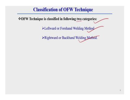
Now, we got the idea about different combustion of different oxy-fuel gases and there we have observed that how much temperature what is the range of temperature generally developed for different combustion of a different fuel gases. And we have observed that where is the application of what types of fuel gases that we already observed. Now, we will discuss about classification of oxy-fuel welding technique.
