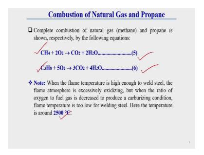
Now, we will discuss about the other fuel gases combustion that is the combustion of natural gas and propane. This equations 5 and 6 generally represent the detailed combustion chemical equation of a first equation represent the methane combustion details and second equation represent the propane combustion chemical equation or chemical reaction.
