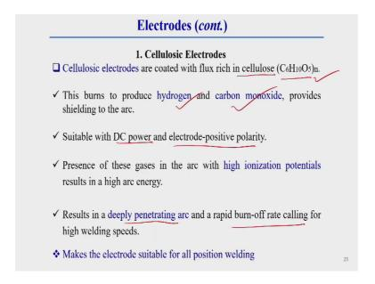
Now, one by one I will discuss in subsequent slide. First of all I will discuss about cellulosic electrode. You see cellulosic electrodes are coated with flux rich in cellulose. So, whatever the flux cover we are using they are generally rich of cellulose is there cellulose is a chain of C6 H10 O5. So, this rich of these composition is there in this electrode. So, when this electrode or a flux burn then this produce hydrogen and carbon monoxide.
