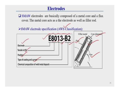
So, the first of all I will discuss about electrode. So, you see generally SMAW process the electrode what I have already told you there is a core metal wire, over this core metal wire there is flux cover. So, you see this is symmetric diagram represent here you see there is a core wire, metal wire through which current is flowing and over this core metal wire there is flux cover; you see the there is flux cover there.
