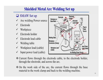
This represent the setup of shielded metal arc welding, this figure represents. Here you see here this is called power source, so, there is a power source. There is you see input power cable or using this power cable also sometimes call input power lead ok; cable is also sometimes called lead. There is a electrode lead cable is there, this is electrode lead
