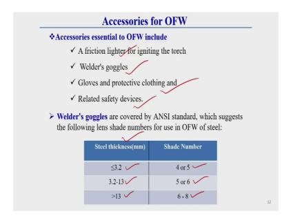
Now, what are the accessories for this oxy-fuel welding technique that also you should know. Here the measure accessories of oxy-fuel welding techniques are for starting the arc, there is required a friction lighter for igniting the torch. Then there is required some welding goggles because whatever the arc is generated this arc can be harmful to eye. That is why they are used for some goggles. So, that goggles also is a accessories of oxy-fuel welding.
