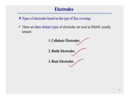
Now, we will discuss about different type of electrode which used in case of shielded metal arc welding process. In case of shielded metal arc welding process there are depending upon the composition of this flux cover, this can be categorized into 3
