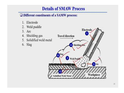
Here the in case of SMAW process there is used a electrode, then you here is a weld puddle, second one is weld puddle, there is a arc, there is shielding gas which is generated due to burning of this coating electrode coated electrode flux. Then, there is slag; slag means after burning of this flux generally it is float over the solidified weld metal and it is solidify, then this is generally called slag and this is generally called solidified weld metal also.
