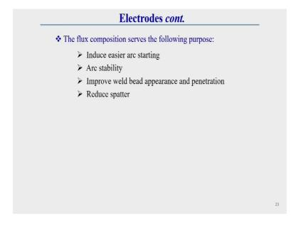
Now, the flux composition serves the following purpose; that means, this flux composition also induce easier arc starting, this flux composition provide arc stability. It is also improve weld bead appearance and penetration and it also reduce the spatter during welding operation of welding operation.
