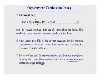
Here rest of the oxygen, whatever the rest of the oxygen are there here, this oxygen generally coming from the surrounding atmosphere. So, here in equation 5, we have seen that there is five molecules of oxygen are there, and two molecules of acetylene are there in this reaction equation.
