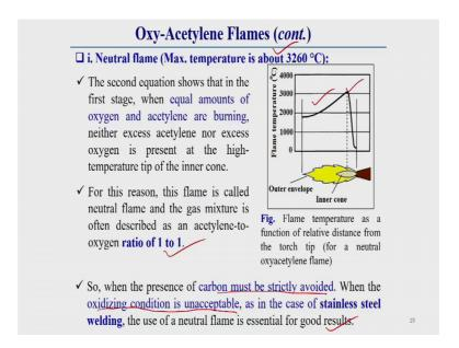
Now, neutral flame so, neutral flame further increase with this reduce flame, if we further increase the what it is called oxygen content, then what happens it approaches to 1 is to 1. So, once the ratio of oxygen and acetylene is become 1 is to 1, then this flame is called neutral flame. This neutral flame have a temperature, it is about 3260 degree centigrade.
