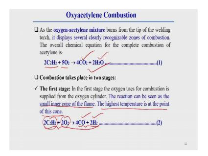
Now, we will discuss first of all combustion of oxy-acetylene gas, then we will discuss about combustion of other fuel gases. So, first of all we will discuss about combustion of oxy-acetylene gases. Here as the oxy-acetylene mixture burn from the tip of the welding torch, it display several clearly recognized zone of combustion.
