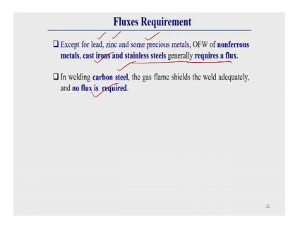
Now, the flux requirement; sometimes flux also required in case of oxy-fuel weldings, except for lead zinc and for some precious metal, oxy-fuel welding of non ferrous metal, cast iron, and stainless steel require a flux. Except for this lead zinc and some precious metal, oxy-fuel welding requires flux. Once that the sum like it can be non ferrous metal, cast iron, stainless steel, flux is required.
