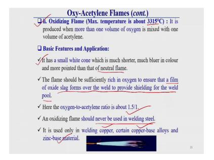
Now, the last categories of oxy-acetylene flame that is called oxidizing flame, here this is oxidizing flame. Here what I have told you, if we increase the oxygen percentage or oxygen proportion, this flame temperature gradually increase. Here the maximum temperature is more than the neutral flame that is 3315 degree centigrade. It is produced when more than one volume of oxygen is mixed with one volume of acetylene. So, here proportion of oxygen is more than the proportion of acetylene gas.
