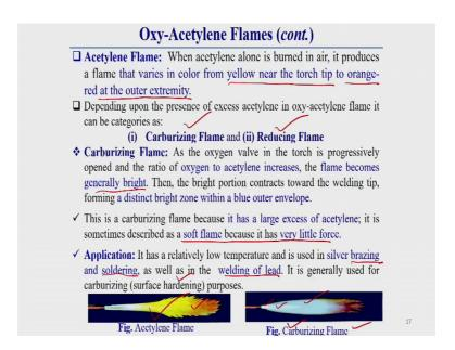
So, first of all I will discuss about acetylene flame. Generally, then acetylene flame that means in this then I will discuss about neutral flame, then I will discuss carburizing flame. So, the acetylene flame, when acetylene alone is burned in air that means, when the arc is started, it produce a flame that varies in color from yellow near the torch tip to
