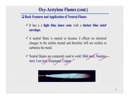
So, this is the basic feature and application of this neutral flame. It has a light generally this is a neutral flame practical neutral flame. Here one things you can say, it has blue inner cone, this is a blue inner cone with a darker blue outer envelope, you see which is the darker blue outer envelope. A neutral flame is named so because, it effects no chemicals changes in the molten metal, and therefore will not oxide or carburize the metal.
