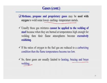
Now, we will discuss about this methane, propane and proprietary gas. This methane generally propane and proprietary gases may be used with oxygen to weld some generally this has a application for some low melting temperature metal. It is used for very low melting temperature metal especially like aluminum, manganese, then lead like bronze, this types of metal generally can be welded by this types of gaseous.
