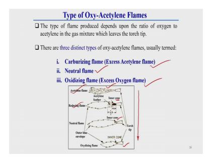
Now, we will go for categories of oxy-acetylene flame. The type of flame produce depends on what I have already discuss that means, depends upon the ratio of oxygen to acetylene in the gas mixture, which generally leaves from the torch tip that means, whatever the gas mixture is coming out from the torch tip, whatever the ratio of this oxygen and fuel gases or acetylene gases, depending upon that ratios generally.
