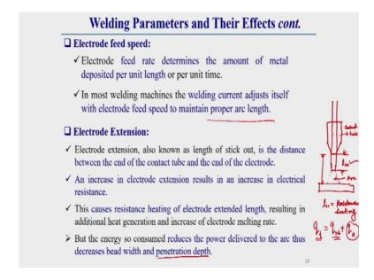
Now, we will see what is the effect of electrode feed a speed? Then, we will go for what is the effect of electrode extension and finally, we will discuss, what is the effect of electrode diameter effect?
