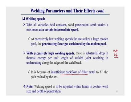
Now, why this is happened because at excessively, because if we decrease the speed again and again. So, at excessively low welding speed what happens, the arc a strike a large molten pool, definitely what happens if the welding speed will be low, then what happens volume of molten material will be high at a particular location.
