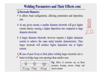
Now, the last parameter that is called electro diameter, which have also effect this electrode extension diameter also significant effect on bead configuration, penetration, and deposition rate. Why, we generally electrode diameter means; towards the electrolyte, this is one electrode, if the electrode diameter, this is this is another electrode diameter. So, here one things you should remember.
