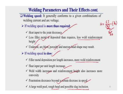
Now, we will go what is the effect of welding speed, this welding speed is the generally very interesting or important parameter, which generally represent; that means, how much heat will be supplied per unit length, that we can this idea we can get from welding speed. How you can you can represent this thing, that I have already discussed you that is the heat supply per unit length is equal to voltage into current divided by welding speed.
