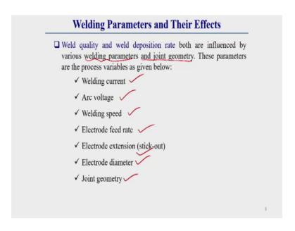
Generally, here one things you keep it in mind, weld quality and weld deposition rate, both are influenced by generally various welding parameters and joint geometry. This generally this weld quality and deposition rate is depends on different welding parameters and another things join geometry. About joint geometry generally I have
