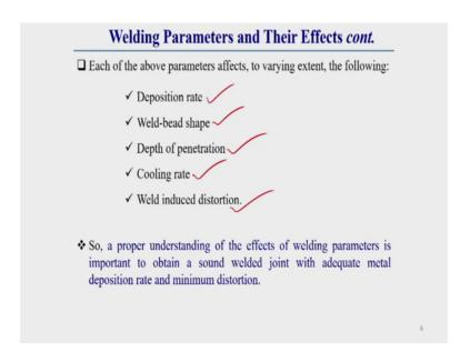
So, before going to welding current generally whatever the parameter I have shown above, this parameter generally affect the following generally, what is the effect of this parameters if it is varying. It is generally these parameters effects the deposition rate, it is effects on weld bead shape, it is effect on depth of penetration, it is effects on cooling rate, and it is effects on weld induced distortion.
