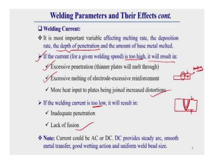
So, from here itself you get the idea; that means, current has is the most important variable generally here. The V generally affecting the melting rate, the deposition rate, the depth of penetration, and the base material melted. So, the amount of base metal melted. So, here one things you keep it in mind this current is the most important variable here.
