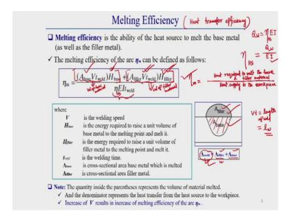
So, last class I have already discuss about heat source efficiency, there we observe that the rate source efficiency is the ratio between the heat in arc; that means, heat supplied to arc by heat by power source. That means, arc heat divided by; that means, heat transfer from arc to work piece; that means, work piece divided by work piece heat.
