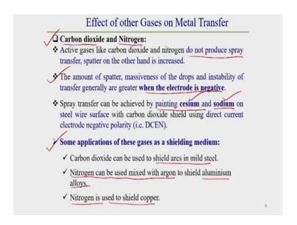
Now, we will discuss about the other gases also. So, generally argon and helium gas this two different inert gas generally used as shielding medium for generally CMAW process or MIG welding process or we can say most of the consumable as well as non-consumable types of electrode or electrode welding process. But, what happens sometimes some other gases also used as a shielding gas that gases generally is not inert
