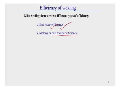
So, that is why generally in case of welding there is two different types of efficiencies used: one is called heat source efficiency another one is called melting or heat transfer efficiency. These heat transfer efficiency generally used in case of net heat transfer actually. So, to know this heat transfer efficiency first of all we should know heat source efficiency.
