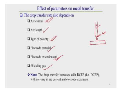
So, we got the idea about melting rate; that means, how the melting rate dependent. Now we will see this metal transfer and its type, what are the parameters generally affected this two; that means, type of metal transfer and a metal transfer rate how its affected by different operating parameters of welding process.
