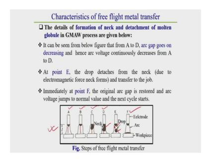
Now, here we will see how the means drop transfer occurs and how it is current voltage characteristic in case of free flight metal transfer, that first we will observe after that we will go for other categories also how the characteristics is look like.
