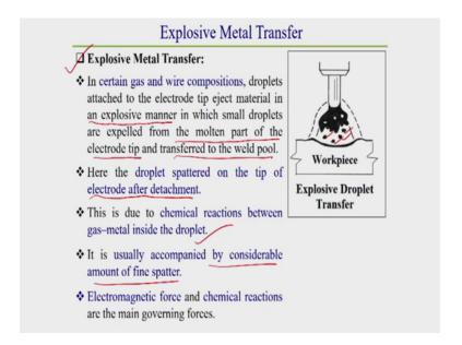
Then the another types of free flight metal transfer is called Explosive metal transfer, in certain gas and wire compositions droplets attached to the electrode tip is material in an explosive manner. Here the molten droplet which is ejecting from the electrode which explosive manner, in which a small droplets are expelled from the molten part of the electrode tip and transferred to the weld.
